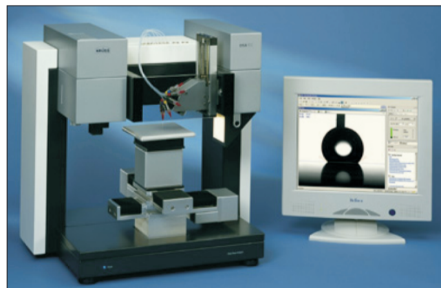
FIG. 6 DROP ANALYSER FOR MEASURING CONTACT ANGLE AND HENCE SURFACE ENERGY
