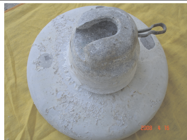
FIG. 5 RTV COATED PORCELAIN DISC INSULATOR AT THE END OF 4600 HOURS OF AGEING TEST
