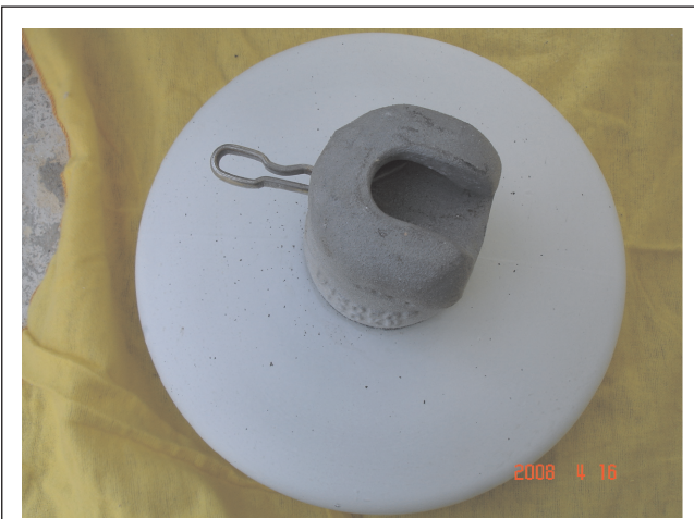
FIG. 2 RTV COATED PORCELAIN (CAP VIEW) DISC INSULATOR BEFORE AGEING TEST
