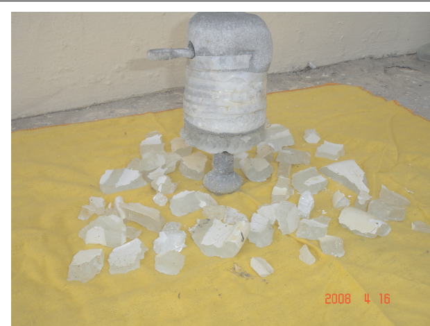
FIG. 6 RTV COATED GLASS DISC INSULATOR (SHATTERED PIECES) AT THE END OF 2600 HOURS OF AGEING TEST
