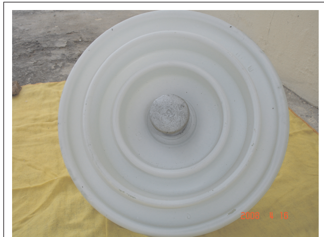
FIG. 3 RTV COATED GLASS (PIN VIEW) DISC INSULATOR BEFORE AGEING TEST
