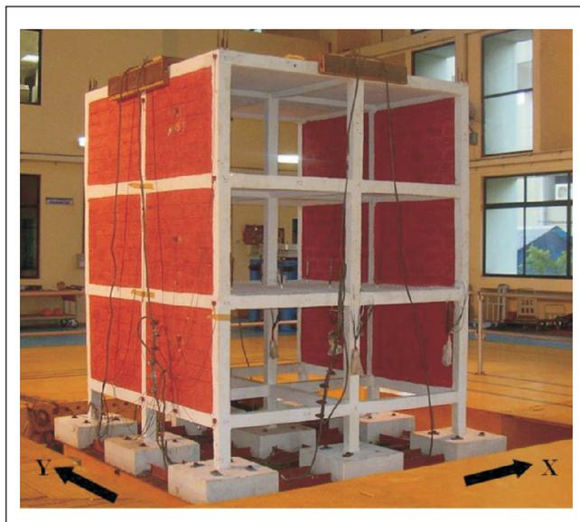
FIG. 7 FIRST 3D MODEL ON SHAKE TABLE
