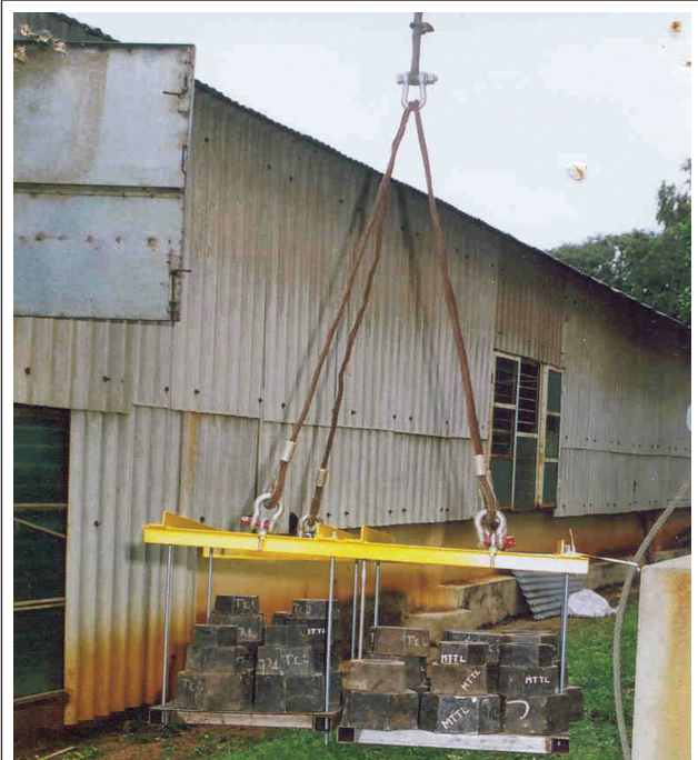
PC WORK STATION TABLE UNDER TEST AND MATERIAL HANDLING FRAME UNDER TEST
