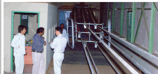
\pm 800 kV HVDC SINGLE 'Y' \pm 800 kV HVDC TRIPLE TENSION SUSPENSION INSULATOR STRING WITH SIX BUNDLE CONDUCTOR CONFIGURATION. TESTED FOR NGK, JAPAN
