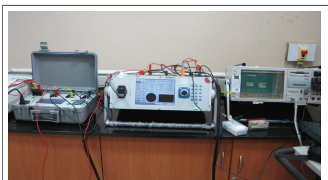
SET UP FOR CALIBRATING 0.05 CLASS PORTABLE REFERENCE METER
