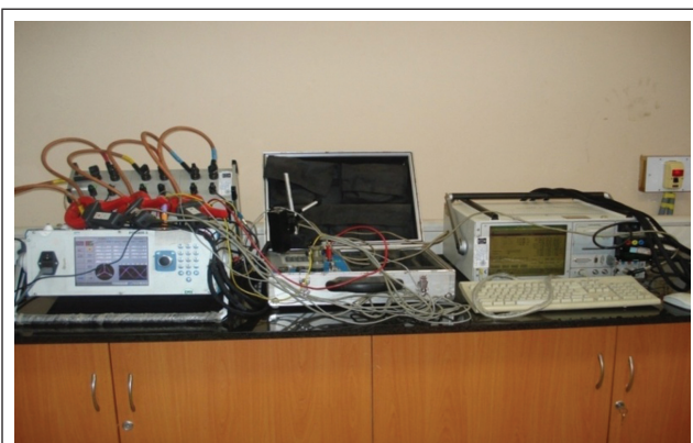
SET UP FOR CALIBRATING THREE PHASE ACCUCHECK MAKE CALLIBRATOR
