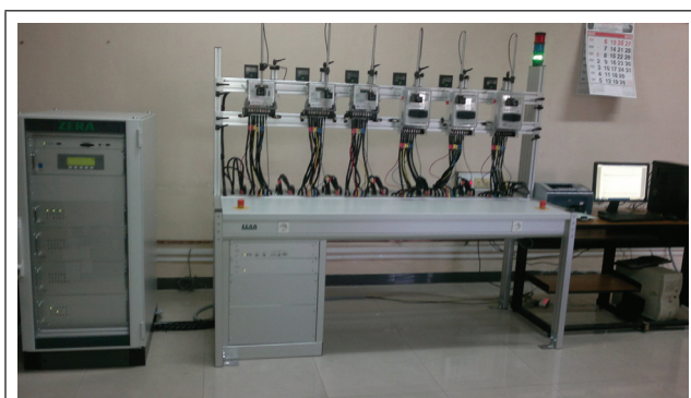
6-POSITION FULLY AUTOMATIC TEST BENCH FOR ENERGY METER TESTING
