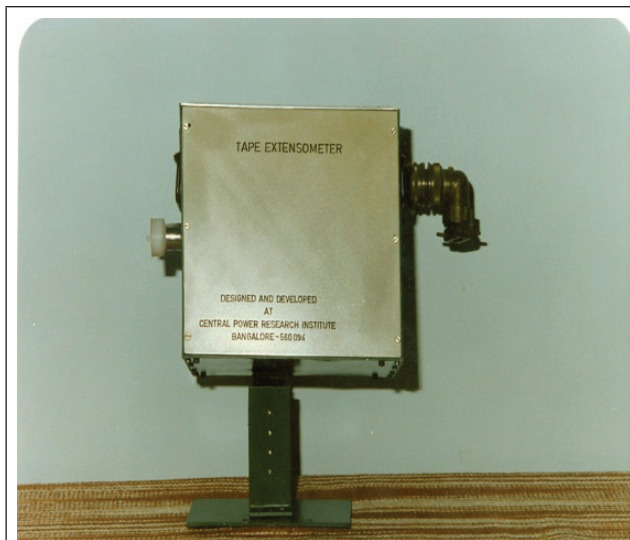
TAPE EXTENSOMETER USED IN 'POWERED SUPPORT CHARACTERISTICS RECORDER' FOR DISPLACEMENT MEASUREMENT
