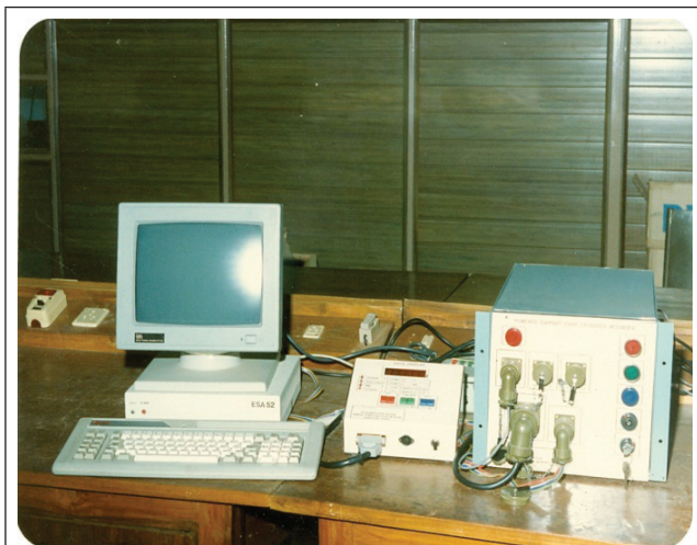
DATA DOWNLOADING INTO PC FROM 'POWERED SUPPORT CHARACTERISTICS RECORDER'
