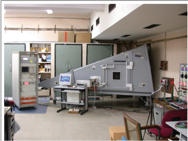
GTEM CELL (80 MHz TO 1000 MHz AT 10 V/mtr.) FOR HF FIELD TEST
