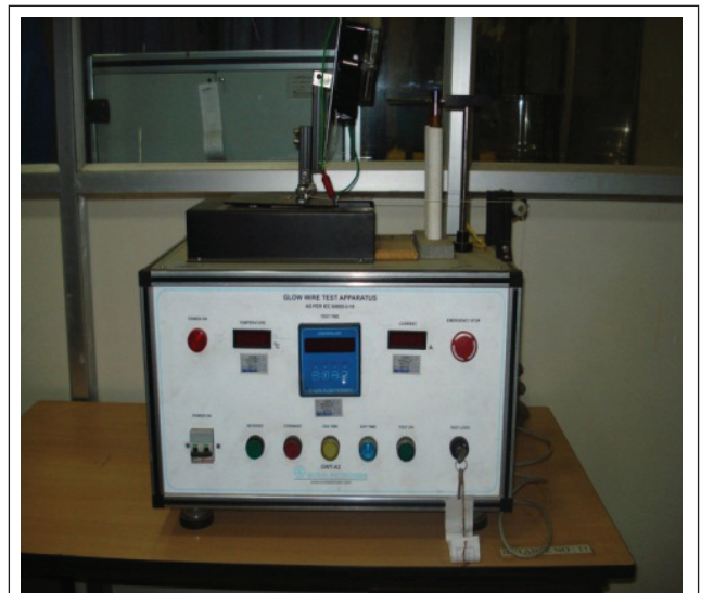
GLOW WIRE TEST SETUP
