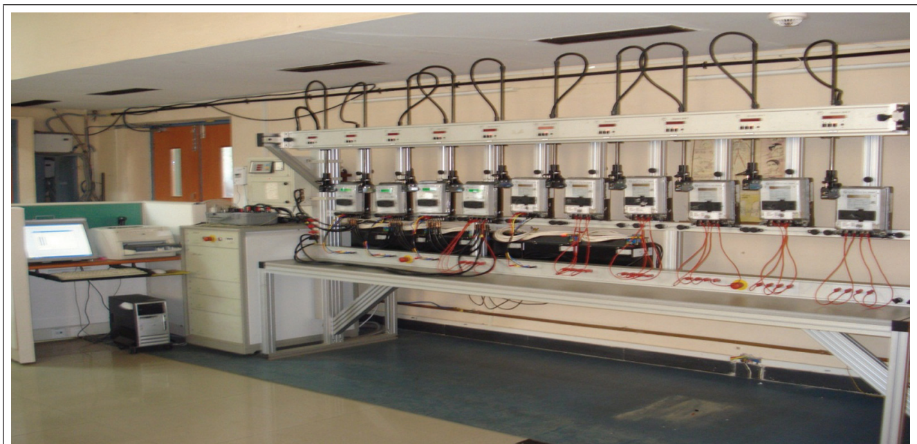
10-POSITION FULLY AUTOMATIC TEST BENCH FOR ENERGY METER TEST BENCH
