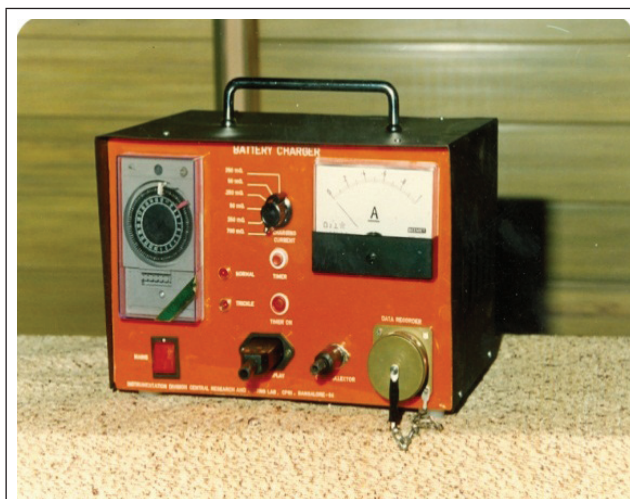
BATTERY CHARGER USED IN 'POWERED SUPPORT CHARACTERISTICS RECORDER' FOR CHARGING INTRINSICAL SAFE RECHARGEABLE BATTERIES
