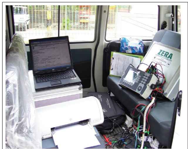
MOBILE ENERGY METER TESTING LABORATORY (INSIDE VIEW)
