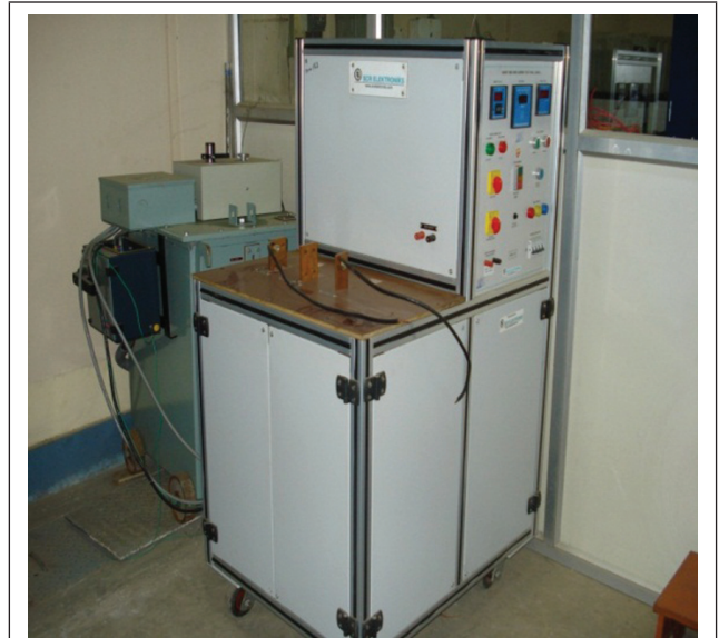
SHORT TIME OVERCURRENT SET UP
