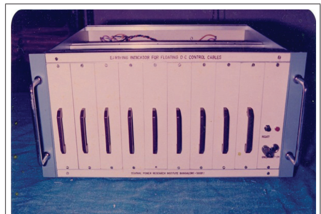
INDICATOR FOR FLOATING DC CONTROL CABLES
