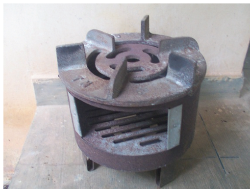
CPRI DESIGNED WOOD BURNING STOVE 1981
