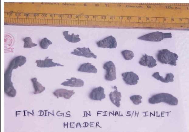
FOREIGN ENTRAPPED OBJECTS FOUND DURING FORCED OUTAGE INVESTIGATION OF BOILER TUBE FAILURE (STEAM STARVATION)
