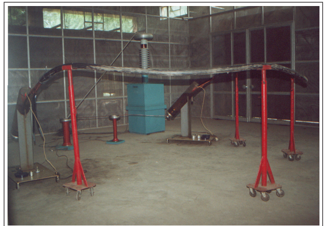
PARTIAL DISCHARGE TEST SET UP
