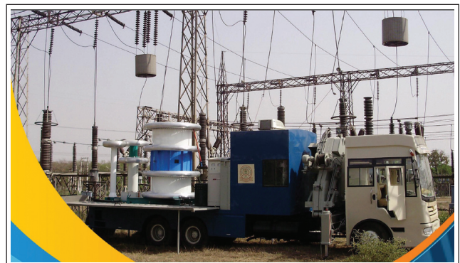
MOBILE TEST FACILITY FOR CTs AND CVTs
