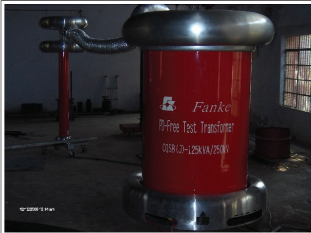
250 kV 125 kVA PD FREE TRANSFORMER
