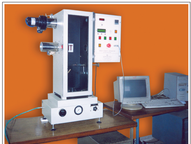
100 kV SMOKE DENSITY TEST APPARATUS
