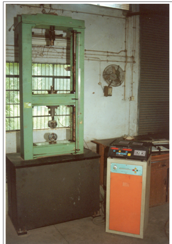
UNIVERSAL TESTING MACHINE (FOR TENSILE STRENGTH TEST AND ELONGATION TEST)
