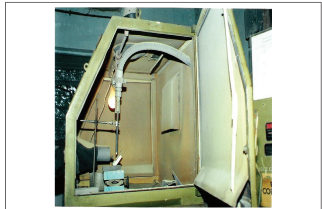
JET EROSION TEST SETUP
