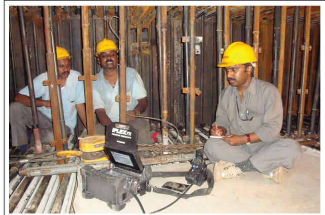
FIBROSCOPIC INSPECTION OF LTRH TUBES
