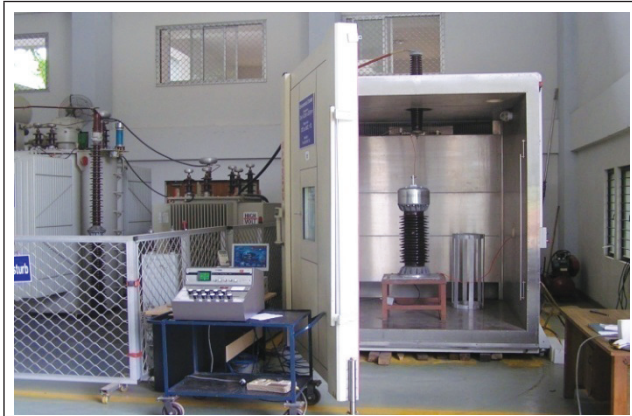
FIG. 18 A VIEW OF ARRANGEMENT FOR CVT TESTING
