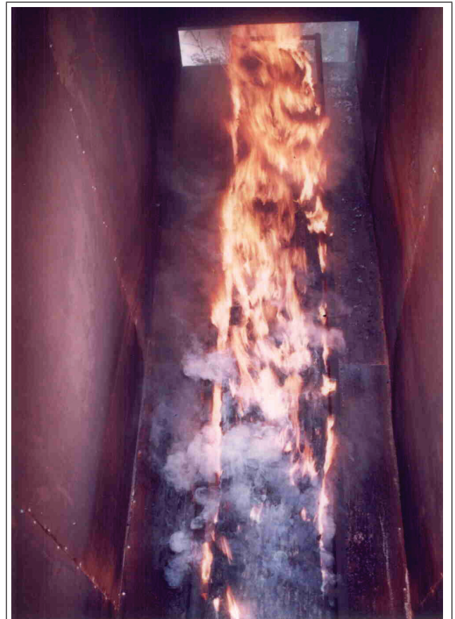
FIG. 18 FLAMMABILITY TEST ON BUNCHED CABLES
