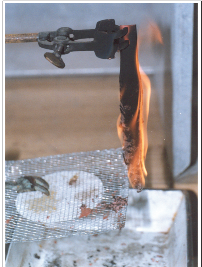
FIG. 17 FLAMMABILITY TEST ON PLASTICS
