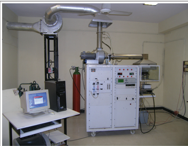
FIG. 20 A VIEW OF CONE CALORIMETER TEST SET UP
