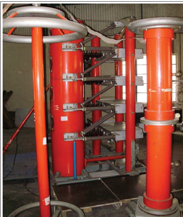
FIG. 11 500 kV, 15 kJ IMPULSE GENERATOR WITH DIVIDER
