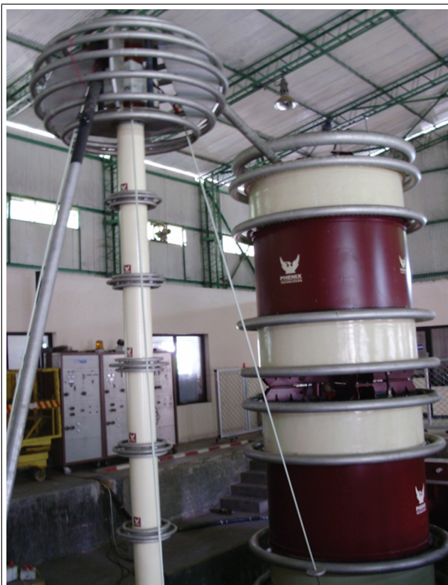
FIG. 12 600 kV, SERIES RESONANT TRANSFORMER JOINTS
