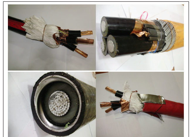
FIG. 22 TYPICAL CABLES TESTED
