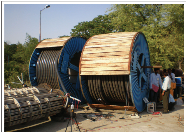
A VIEW OF ARRANGEMENT FOR TESTS ON POWER CABLES IN PROGRESS
