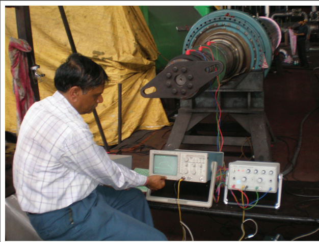
A VIEW OF RSO TEST ON GENERATOR ROTOR IN PROGRESS
