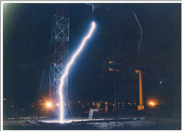
FIG. 8 FLASHOVER OF 25 m ROD-PLANE GAP UNDER SWITCHING IMPULSE
