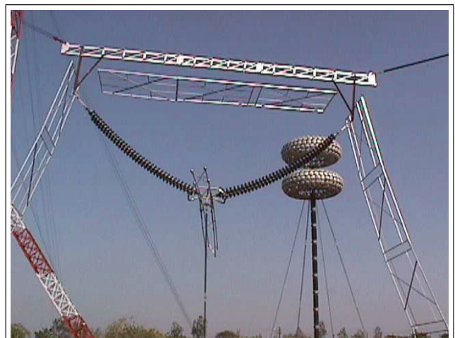
FIG. 5 A VIEW OF 1200 INSULATOR STRING WITH SIMULATED TOWER
