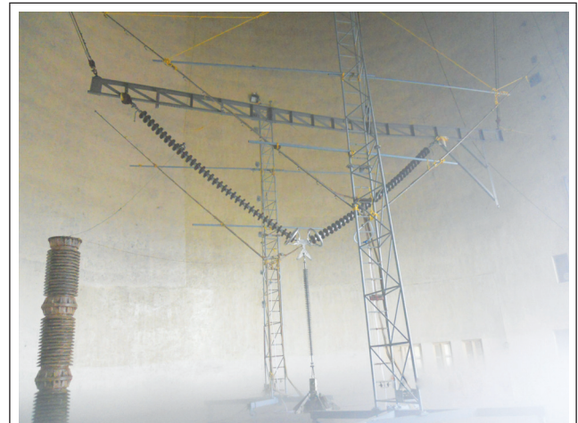
FIG. 37 765 kV SINGLE 'V' INSULATOR STRING UNDERGOING POLLUTION TEST
