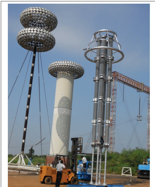
FIG. 30 1200 kV SURGE ARRESTOR
