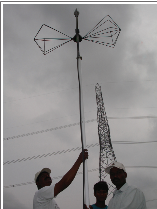
FIG. 22 RIV MEASUREMENTS AT 765 kV TRANSMISSION LINE
