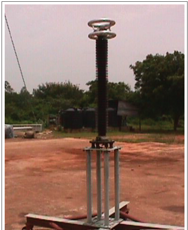
FIG. 11 A VIEW OF 500 kV LIGHTNING IMPULSE VOLTAGE DIVIDER
