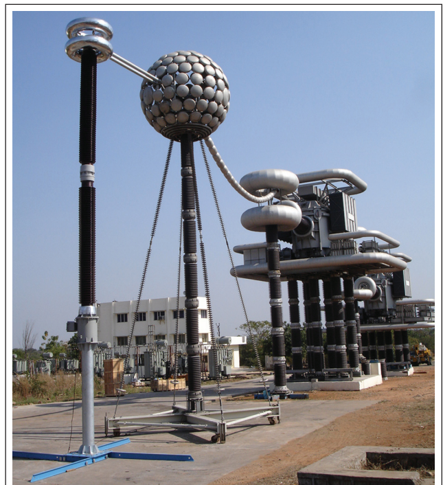
FIG. 27 1200 kV CAPACITOR VOLTAGE TRANSFORMER UNDER TEST IN PF LABORATORY
