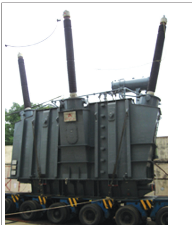
80 MVA, 400/11.5-11.5 kV POWER TRANSFORMER TESTED AS PER IEC 60076-5
