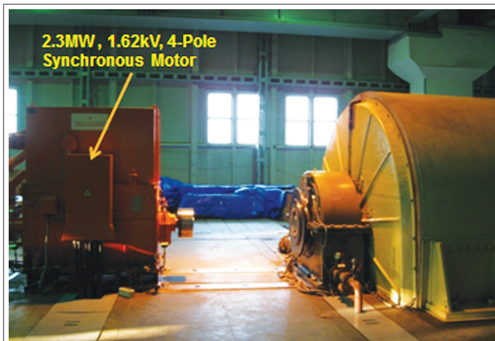
PHOTOGRAPH OF 14 kV, 2500 MVA 50/60 Hz DRIVELESS SHORT CIRCUIT GENERATOR
