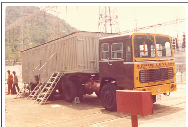
ONE OF THE TWO INSTRUMENTATION TRAILERS OF THE MOBILE FIELD TESTING LABORATORY
