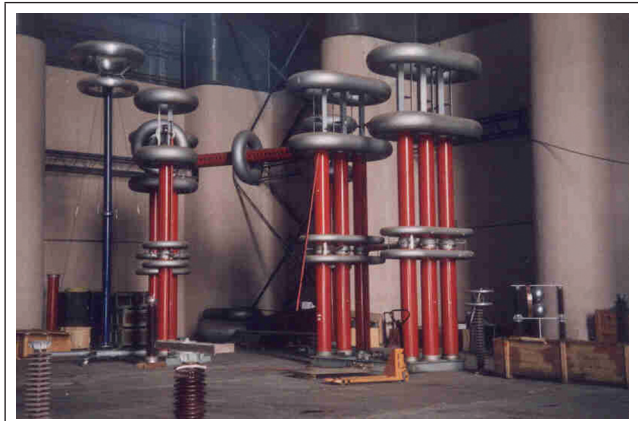
THE 800 kV, 200 MA HIGH-VOLT MAKE DC VOLTAGE SOURCE
