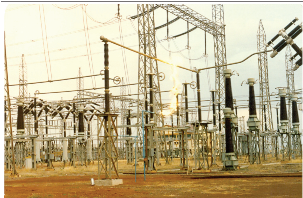
FAULT THROWING ARRANGEMENT AND FAULT ARC DURING MEASUREMENT OF SECONDARY ARC CURRENT
