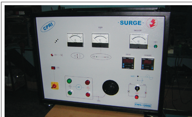
COMBINATION WAVE GENERATOR FOR SURGE IMMUNITY TEST DEVELOPED FOR STDS BHOPAL
