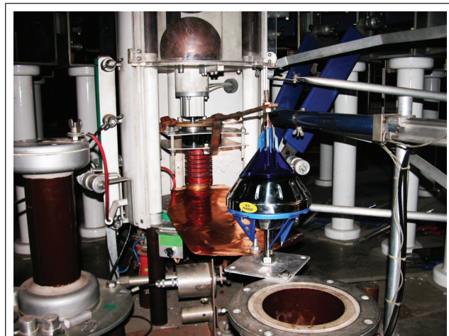
TEST ARRANGEMENT FOR EARLY STREAMER EMISSION LIGHTNING TERMINAL
