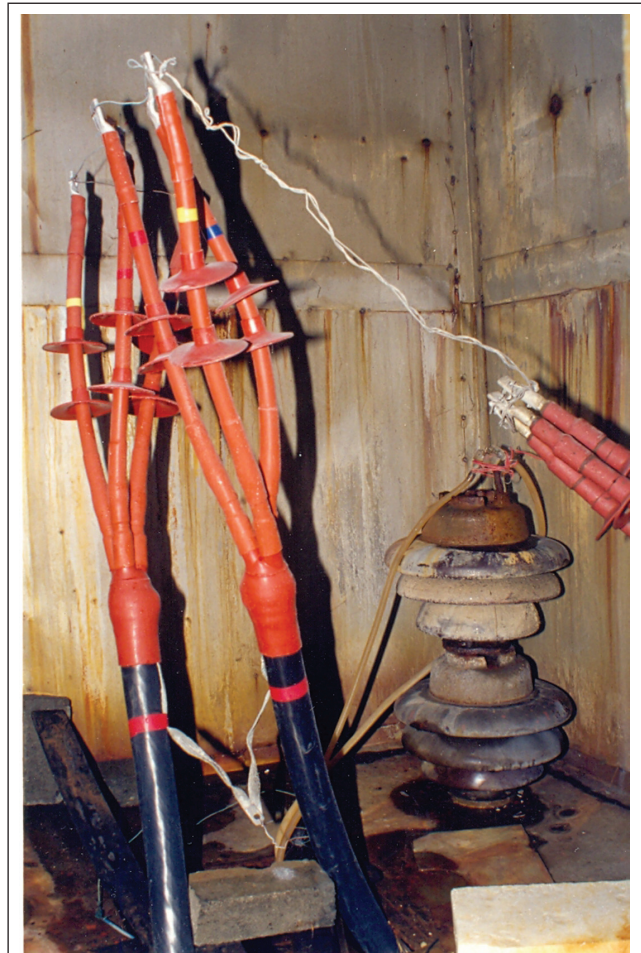
CABLE TERMINATION UNDER 1000 HOUR AGEING TEST
