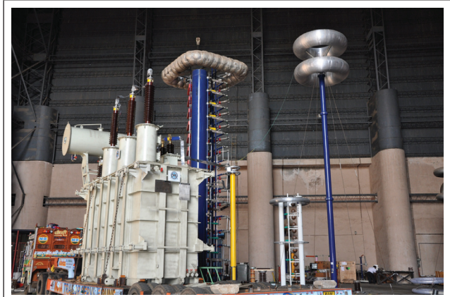
POWER TRANSFORMER UNDERGOING IMPULSE TEST
