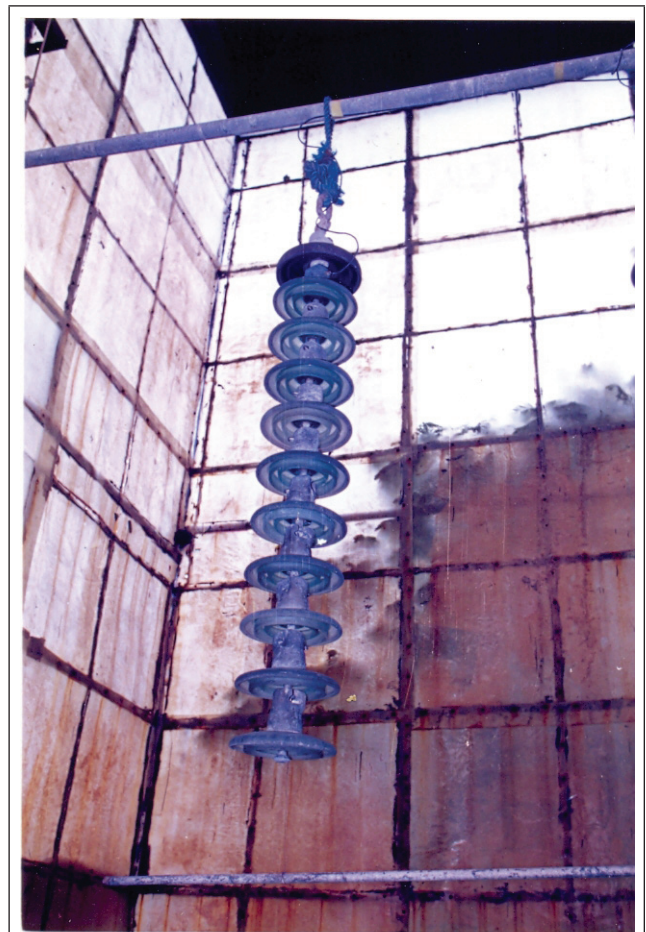
INSULATOR UNDERGOING SALT FOG TEST IN OLD POLLUTION LABORATORY
