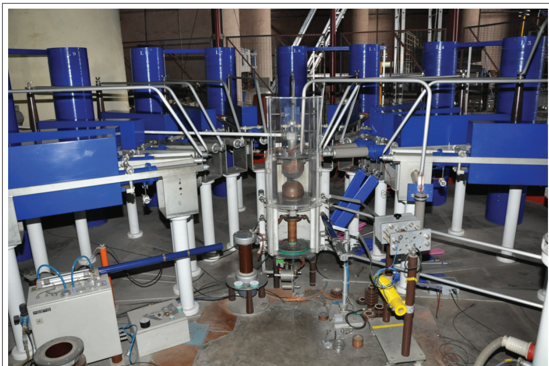
100 kA, 150 kJ IMPULSE CURRENT GENERATOR
