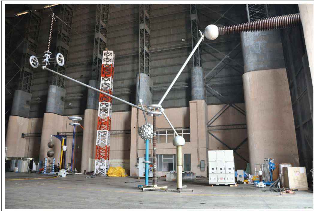
INSULATOR STRING UNDERGOING RADIO INTERFERENCE TEST
