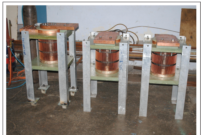
FIG. 23 CO-AXIAL SHUNTS (200 kA)
