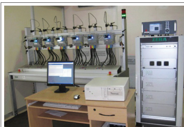
FIG. 12 SIX POSITION TEST BENCH WITH 0.008 CLASS ACCURACY
