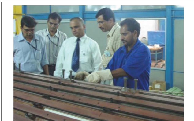
FIG. 22 INSPECTION OF GENERATOR ROTOR AT THE WORKS OF M/S. ALSTOM, VADODARA
