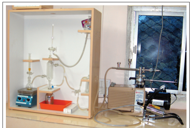
FIG. 15 GAS EXTRACTION SET UP FOR DGA TESTING
