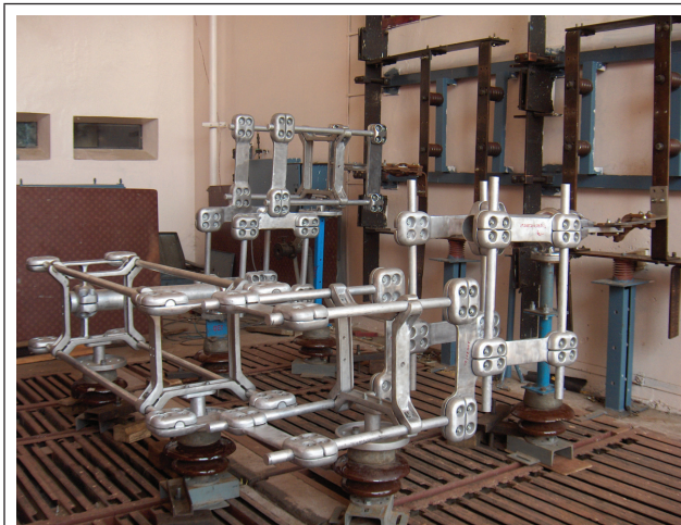
FIG. 17 800 kV, 4000 A POWER CONNECTORS
