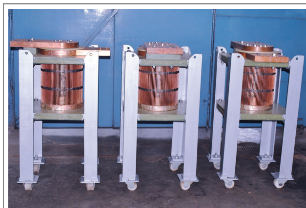
200 kA COAXIAL CAGE TYPE HIGH CURRENT SHUNT
