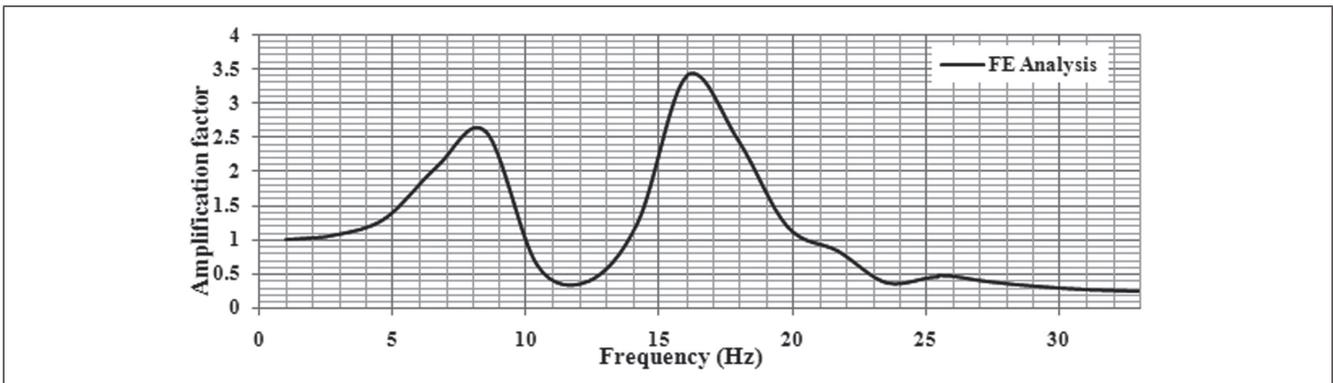
FIG. 5 RESPONSE AMPLIFICATION AT THE BASE OF THE PORCELAIN INSULATOR OF 12 kV CIRCUIT BREAKER IN X-AXIS.
