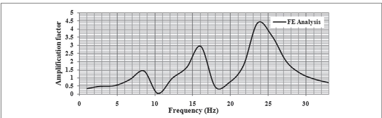
FIG. 6 RESPONSE AMPLIFICATION AT THE BASE OF THE PORCELAIN INSULATOR OF 12 kV CIRCUIT BREAKER IN Y-AXIS.
