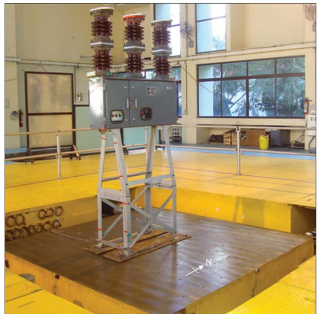
FIG. 1 12 kV CIRCUIT BREAKER WITH SUPPORT STRUCTURE MOUNTED ON TRI-AXIAL SHAKE TABLE.
