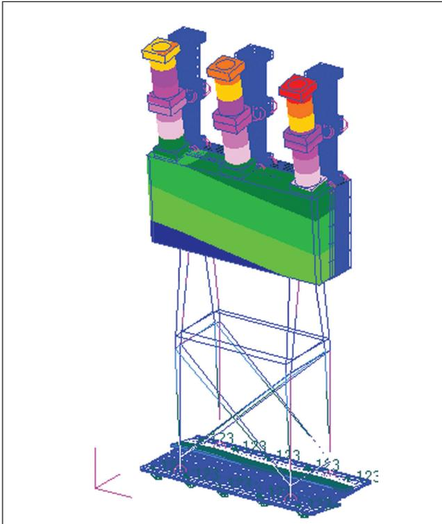
FIG. 2 FIRST MODE OF FINTE ELEMENT MODEL OF 12 kV CIRCUIT BREAKER.
