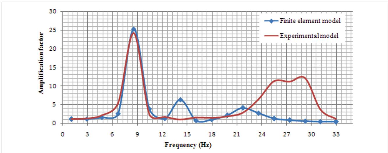
FIG. 4 RESPONSE AMPLIFICATION AT THE TOP OF THE PORCELAIN INSULATOR OF 12 kV CIRCUIT BREAKER IN Y-AXIS.
