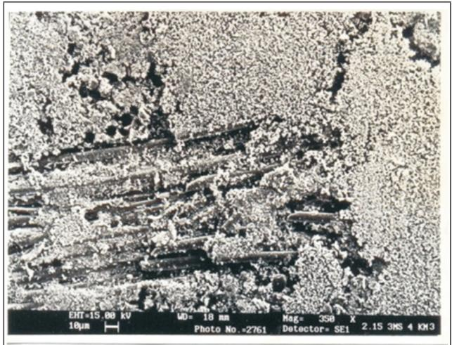
FIG. 5 SLIDE WEAR FEATURES OF G-E SYSTEM FOR 30 N LOAD
