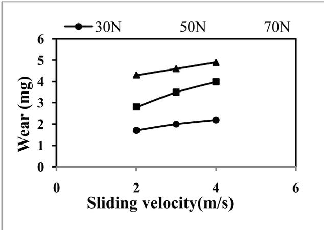
FIG. 1 PLOT OF SLIDE WEAR LOSS V/S SLIDING VELOCITY FOR G-E SYSTEM
