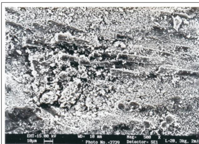
FIG. 8 SLIDE WEAR FEATURES OF G-E + G SYSTEM 30 N LOAD
