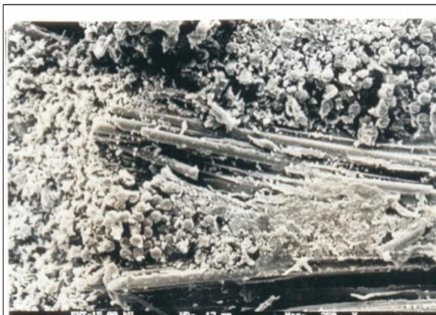
FIG. 7 SLIDE WEAR FEATURES OF G-E SYSTEM FOR 70 N LOAD
