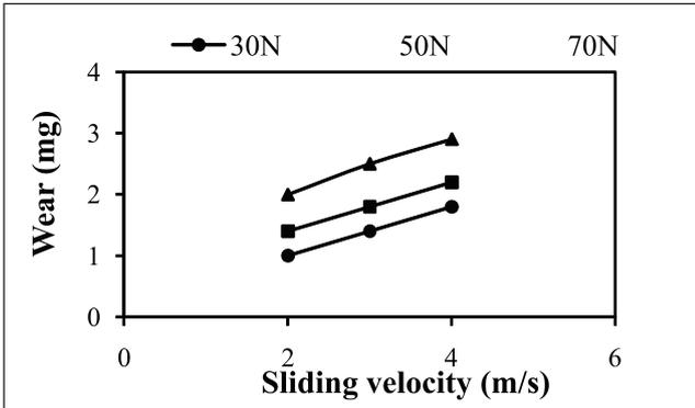
FIG. 2 PLOT OF SLIDE WEAR LOSS V/S SLIDING VELOCITY FOR G-E + G SYSTEM
