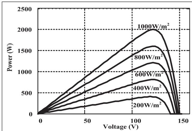
FIG. 2 (A) POWER-VOLTAGE CHARACTERISTICS OBTAINED FROM THE PANEL-A
