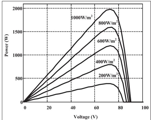
FIG. 3 (A) POWER-VOLTAGE CHARACTERISTICS OBTAINED FROM THE PANEL-A
