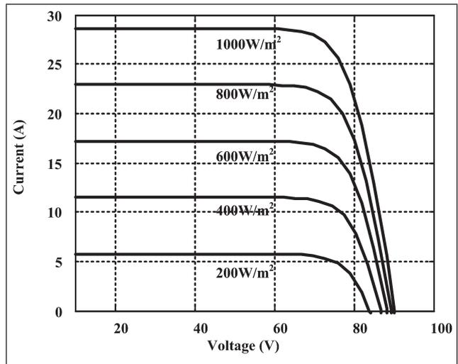
FIG. 3 (B) CURRENT-VOLTAGE CHARACTERISTICS OBTAINED FROM THE PANEL-B
