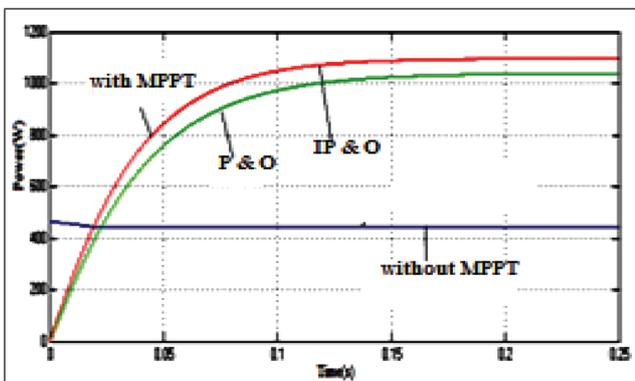
FIG. 13 POWER COMPARISON OF P & O AND IP & O
