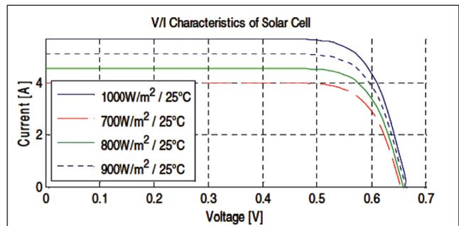
FIG. 9 V/I CURVES OF SOLAR CELL AT DIFFERENT IRRADIATION LEVELS
