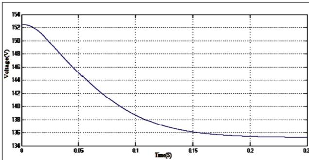
FIG. 11 PV ARRAY OUTPUT VOLTAGE FOR IP & O
