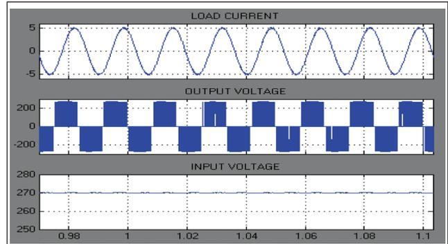
FIG. 8 OUTPUT LOAD CURRENT, OUTPUT VOLTAGE AND INPUT VOLTAGE OF ZSI
