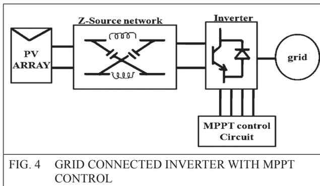
FIG. 4 GRID CONNECTED INVERTER WITH MPPT CONTROL
