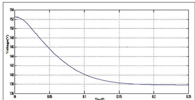
FIG. 9 PV ARRAY OUTPUT VOLTAGE FOR P & O
