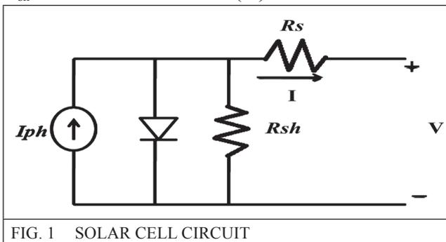
FIG. 1 SOLAR CELL CIRCUIT
