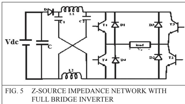
FIG. 5 Z-SOURCE IMPEDANCE NETWORK WITH FULL BRIDGE INVERTER
