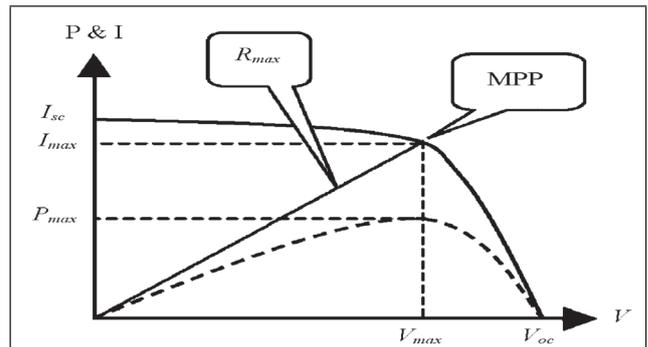
FIG. 3 GENERAL CHARACTERISTIC CURVES OF SOLAR ARRAY
