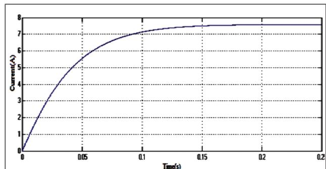
FIG. 10 PV ARRAY OUTPUT CURRENT FOR P & O
