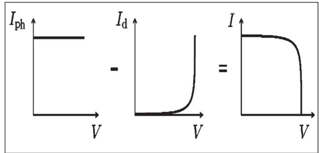
FIG. 2 I-V CHARACTERISTICS OF CELL CURRENT (I)
