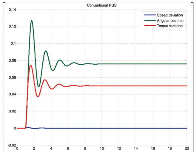
FIG. 9 SYSTEM RESPONSE FOR A 5% CHANGE IN MECHANICAL INPUT WITH CPSS
