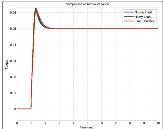
FIG. 13 TORQUE VARIATION FOR 5% CHANGE IN MECHANICAL INPUT FOR DIFFERENT OPERATING CONDITIONS
