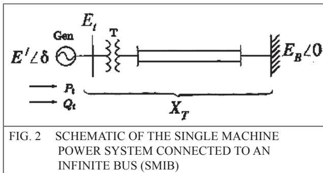
$$\Delta T_e = \frac{\partial T_e}{\partial \delta} \Delta \delta = \frac{E' E_B}{X_T} \cos \delta (\Delta \delta) \quad \dots(2)$$
