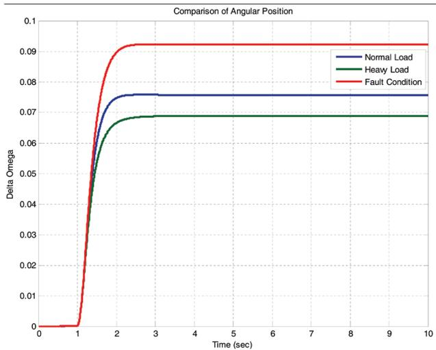
FIG. 11 ANGULAR POSITION PLOT FOR 5% CHANGE IN MECHANICAL INPUT FOR DIFFERENT OPERATING CONDITIONS
