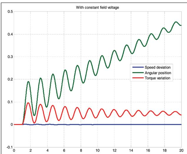
FIG. 7 SYSTEM RESPONSE FOR A 5% CHANGE IN MECHANICAL INPUT WITH CONSTANT FIELD VOLTAGE
