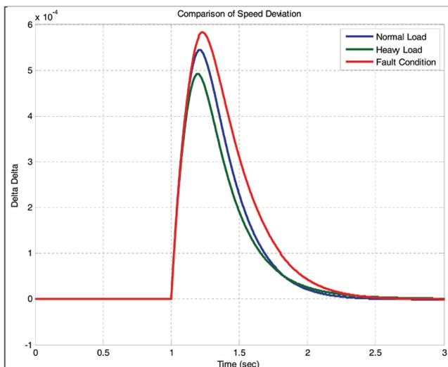
FIG. 12 SPEED DEVIATION PLOT FOR 5% CHANGE IN MECHANICAL INPUT FOR DIFFERENT OPERATING CONDITIONS
