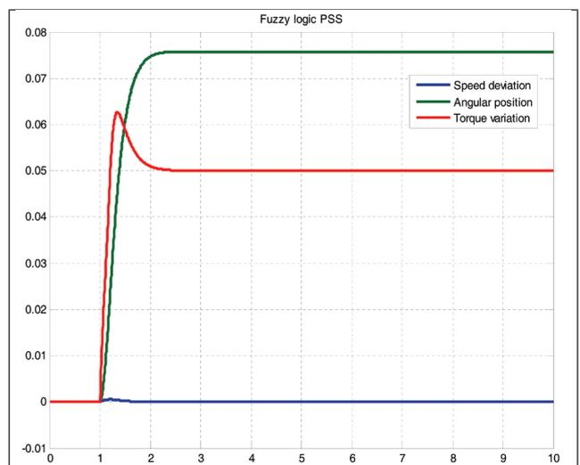
FIG. 10 SYSTEM RESPONSE FOR A 5% CHANGE IN MECHANICAL INPUT WITH FL PSS FOR NOMINAL LOAD
