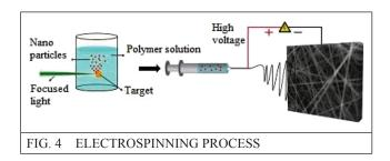
In this process, the polymer solution is pushed through a needle at a constant speed by controlling a syringe pump and a high voltage DC source is used to electrify the polymer solution.
