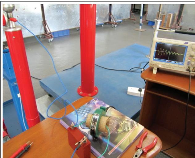
FIG. 3 (A) EXPERIMENTAL SETUP FOR SHORT CIRCUIT DISCHARGE ON A 10NF, 20KV CAPACITOR
