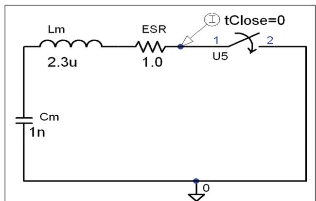
FIG. 4 (C) EQUIVALENT CIRCUIT OF MARX GENERATOR DURING SHORT CIRCUIT DISCHARGE
