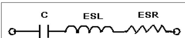
FIG. 1 EQUIVALENT CIRCUIT OF A CAPACITOR
