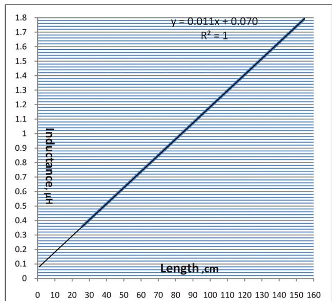
FIG. 3(D) GRAPH SHOWING INDUCTANCE VERSUS DISCHARGE PATH LENGTH OF 10NF, 20KV CAPACITOR
