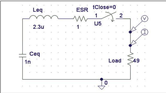
FIG. 5 (A) EQUIVALENT CIRCUIT OF MARX WITH MATCHED LOAD
