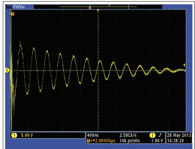
FIG. 4 (B) SHORT CIRCUIT DISCHARGE CURRENT WAVEFORM OF MARX GENERATOR
