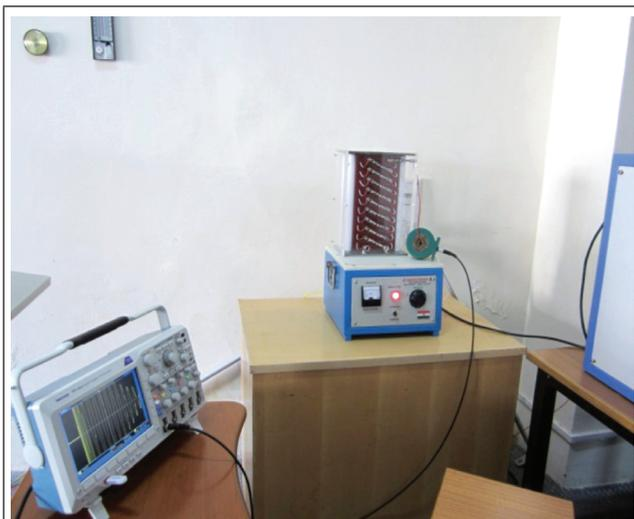
FIG. 4 (A) EXPERIMENTAL SET UP FOR CONDUCTING SHORT CIRCUIT DISCHARGE TEST
