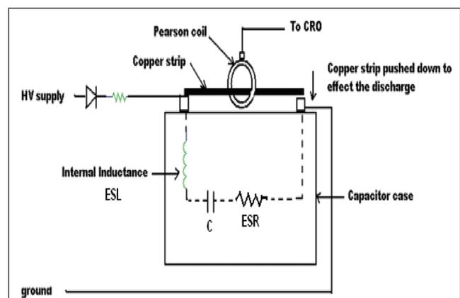
FIG. 2 SCHEMATIC FOR OBTAINING THE DISCHARGE CURRENT TO DEDUCE THE INTERNAL INDUCTANCE
