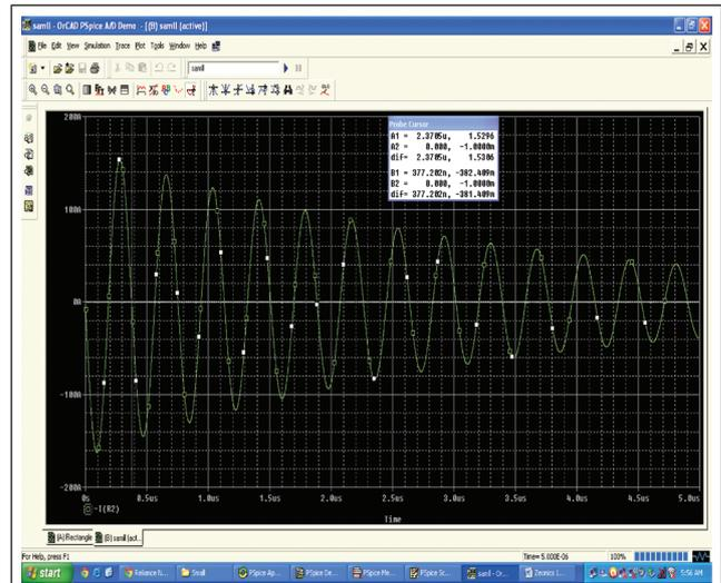
FIG. 3 (C) PSPICE OUTPUT CURRENT WAVEFORM OF 10NF, 20KV CAPACITOR
