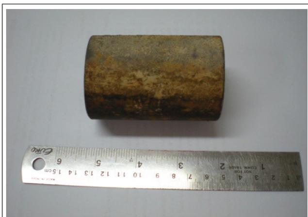
FIG. 1 SLAG DEPOSITED TUBE
