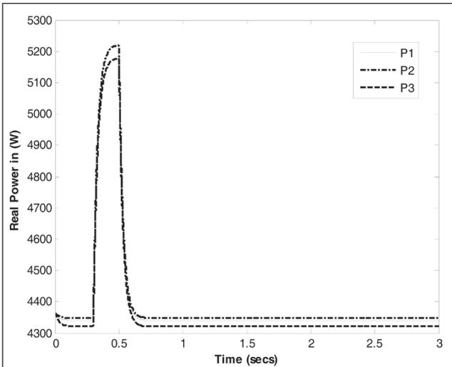
FIG. 8 ACTIVE POWER RESPONSE OF MICRO-SOURCES WITH 3.8 KW OF STEP CHANGE IN LOAD POWER AT BUS 1.
