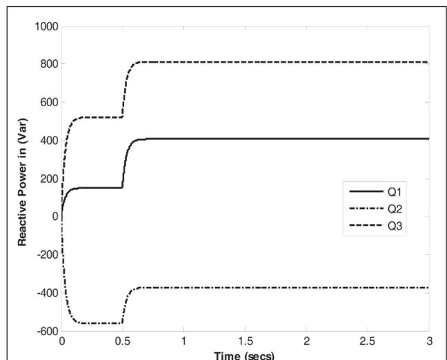
FIG. 11 REACTIVE POWER RESPONSE OF MICRO-SOURCES WITH 16.8 KW AND 12 KVAR RL LOAD STEP CHANGE AT BUS 1.
