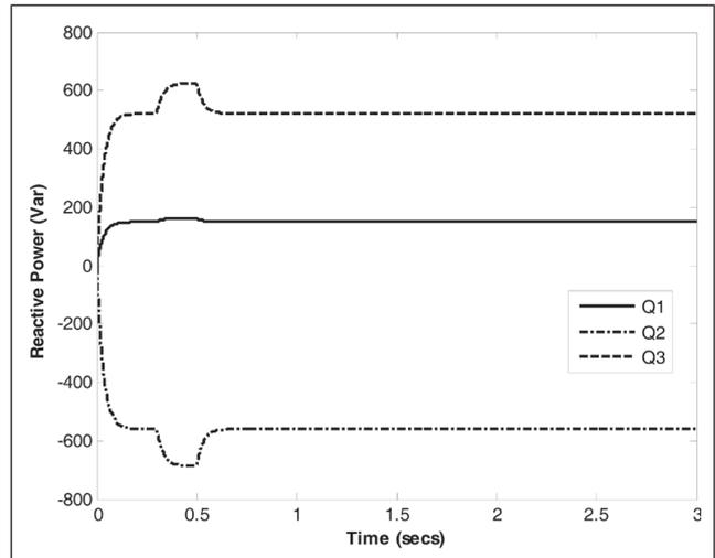
FIG. 9 REACTIVE POWER RESPONSE OF MICRO-SOURCES WITH 3.8 KW OF STEP CHANGE IN LOAD POWER AT BUS 1.
