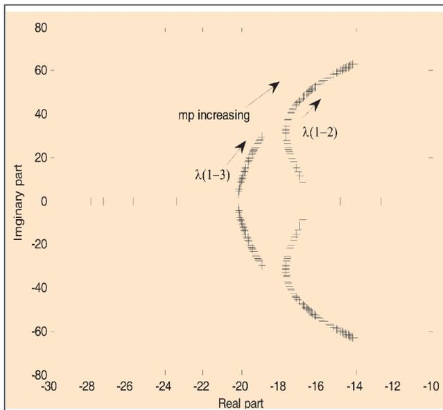
FIG. 6 TRACE OF LOW-FREQUENCY MODES AS A FUNCTION OF REAL POWER DROOP GAIN: 1.57E (0.05% DROOP) \_ M \_ 3.14E
