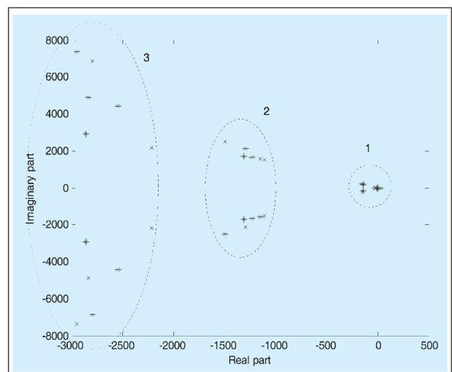
FIG. 5 EIGEN VALUE SPECTRUM OF THE SYSTEM INDICATING VARIOUS MODES.
