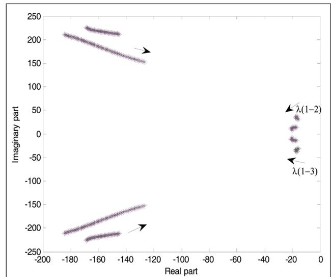
FIG. 7 TRACE OF LOW-FREQUENCY MODES AS FUNCTION OF REACTIVE POWER DROOP GAIN: 3.17E (0.5% DROOP) \_ N \_ 4.8E (8% DROOP)
