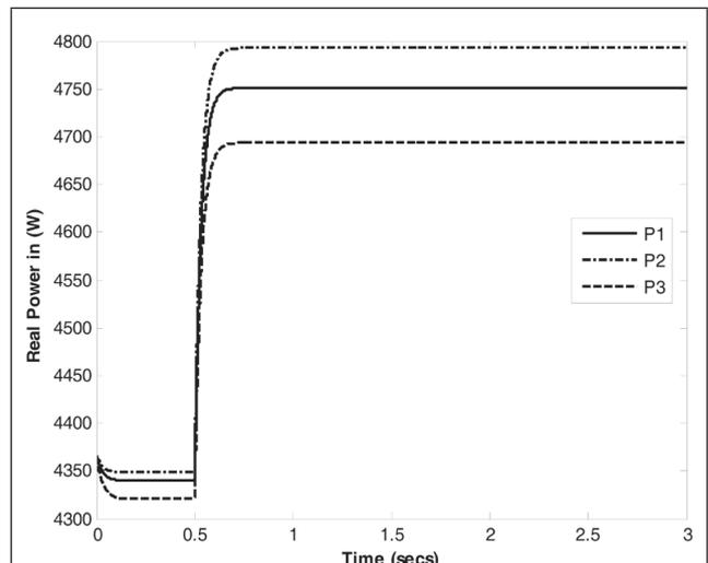
FIG. 10 ACTIVE POWER RESPONSE OF MICRO-SOURCES WITH 16.8 KW AND 12 KVAR RL LOAD STEP CHANGE AT BUS 1.
