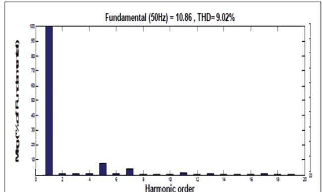
FIG. 12 THD % OF THE INJECTED CURRENT WITH ORDINARY FILTER
