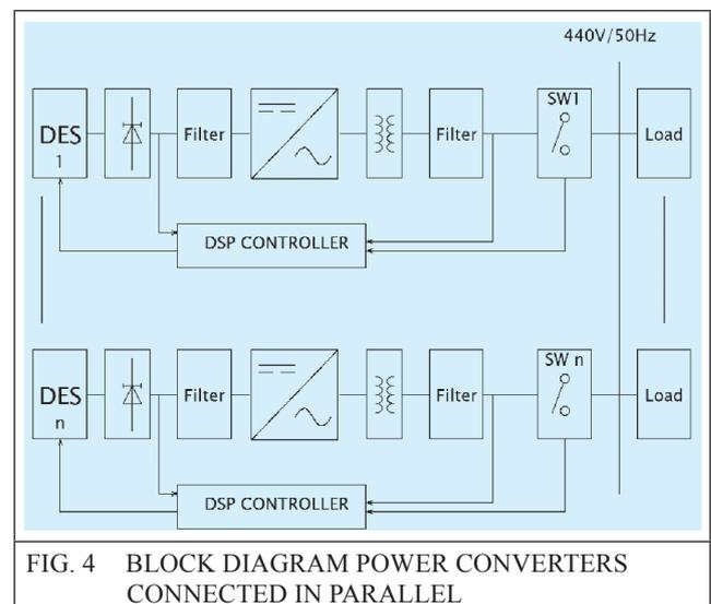
FIG. 4 BLOCK DIAGRAM POWER CONVERTERS CONNECTED IN PARALLEL
