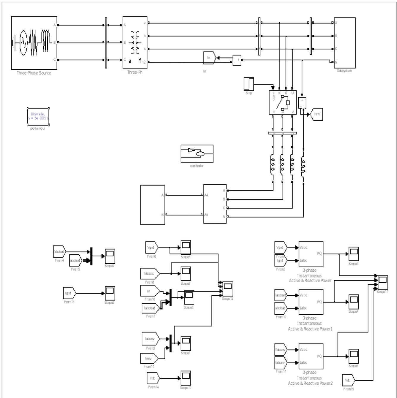
FIG. 8 MATLAB/SIMULINK MODEL FOR THREE PHASE GRID INTERFACING INVERTER
