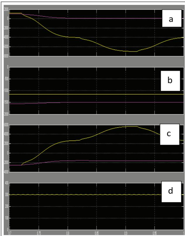
FIG.10 SIMULATION RESULTS: (A) PQ-GRID, (B) PQ-LOAD, (C) PQ-INVERTER, (D) DC-LINK VOLTAGE.
