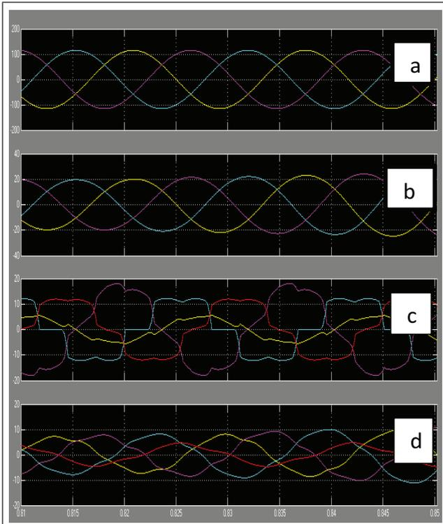
FIG. 9 SIMULATION RESULTS: (A) GRID VOLTAGES, (B) GRID CURRENTS (C) UNBALANCED LOAD CURRENTS, (D) INVERTER CURRENTS
