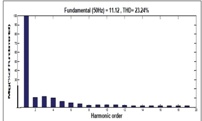
FIG. 11 THD % OF THE INJECTED CURRENT WITHOUT FILTER
