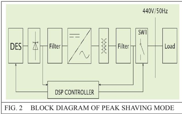
FIG. 2 BLOCK DIAGRAM OF PEAK SHAVING MODE
