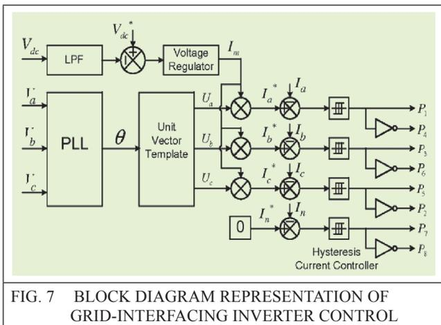
FIG. 7 BLOCK DIAGRAM REPRESENTATION OF GRID-INTERFACING INVERTER CONTROL
