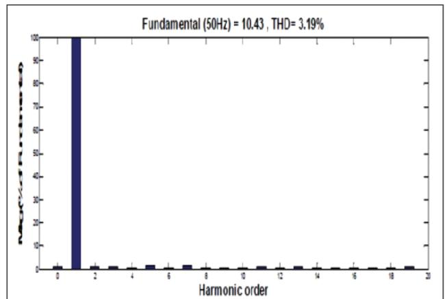
FIG. 13 THD % OF THE INJECTED CURRENT WITH SHUNT ACTIVE FILTER
