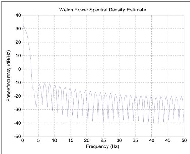
FIG. 7. PSD OF THE TEMPERATURE RISE IN I.M AT DIFFERENT LOAD WITH FAULTY COOLING SYSTEM.
