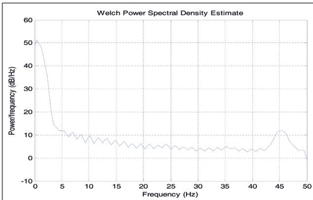
FIG. 3 PSD OF THE CURRENT SIGNATURE
