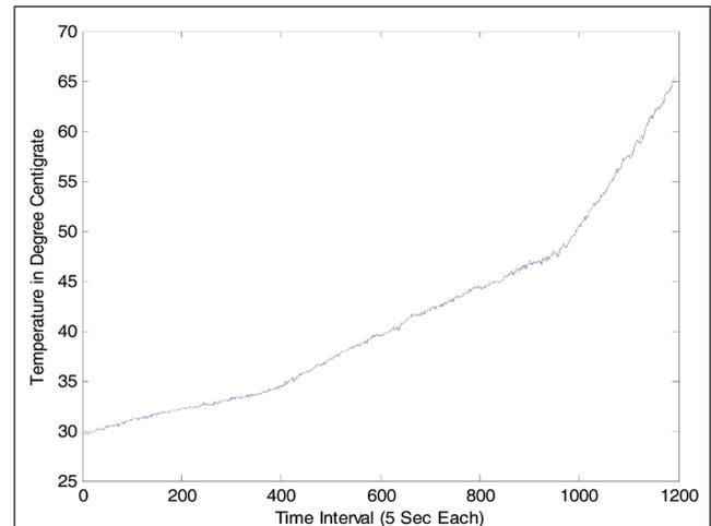
FIG. 6 TEMPERATURE RISE IN I.M AT DIFFERENT LOAD (NO LOAD, QUARTER LOAD, HALF LOAD) WITH FAULTY COOLING SYSTEM.
