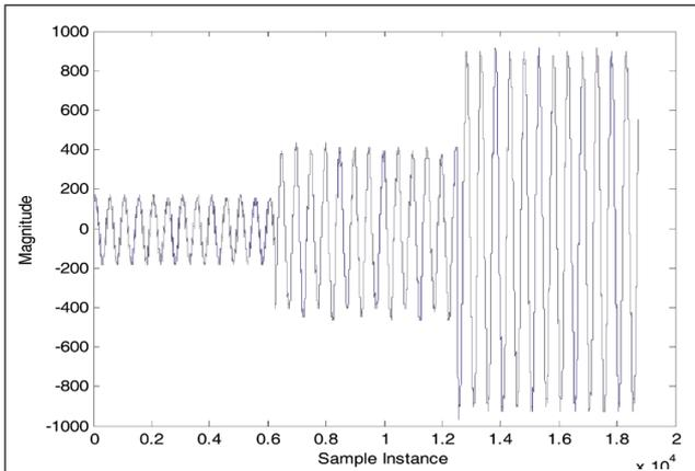
FIG. 2 CURRENT SIGNATURE OF I.M AT DIFFERENT LOAD
