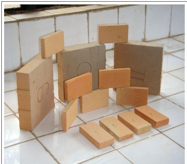
FIG. 9 THERMAL INSULATION REFRACTORY FROM FLY ASH CENOSPHERES
