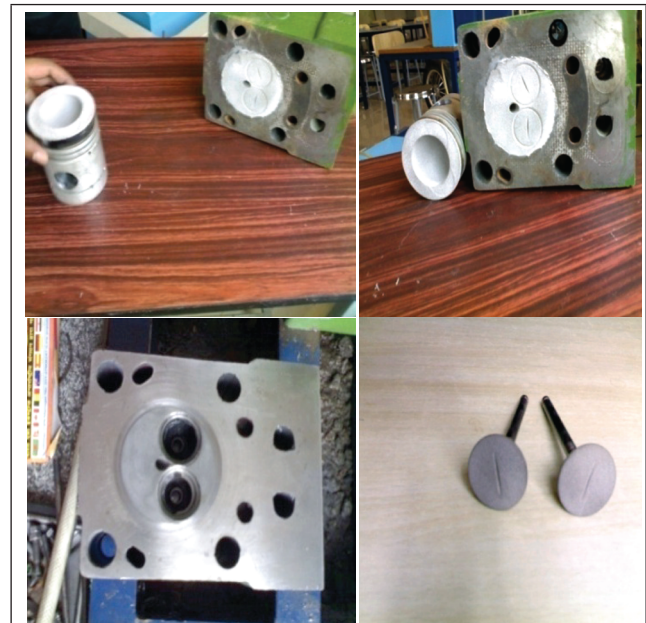
FIG. 3 PHOTOGRAPHIC VIEW OF INSULATED ENGINE COMPONENTS
