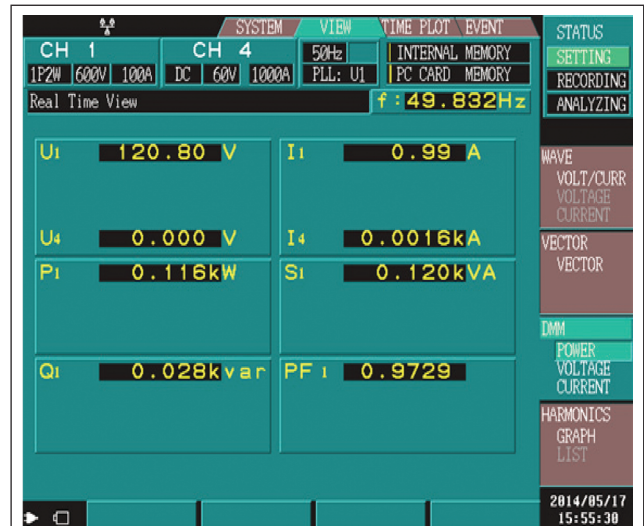
FIG. 13 POWER ANALYZER DISPLAYING POWER FACTOR
