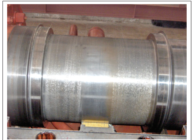
FIG. 7 PITTINGS ON THE SHAFT
