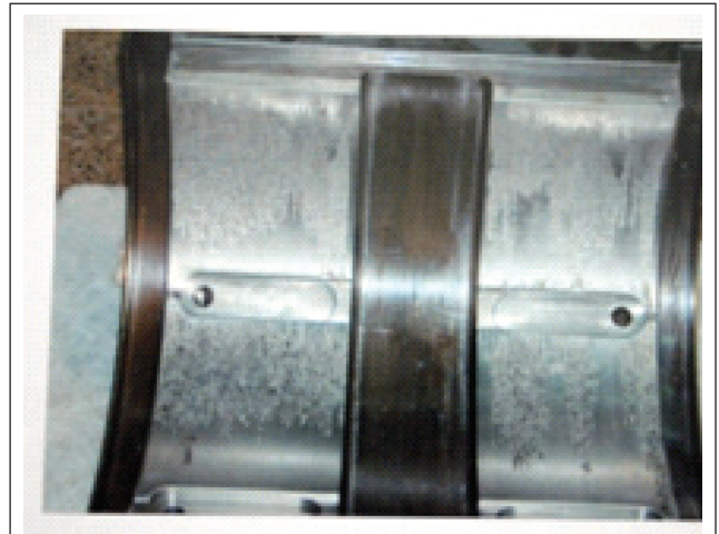
FIG. 6 PITTINGS ON THE BEARING
