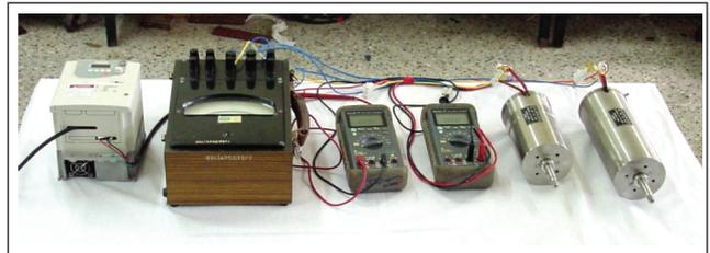
FIG. 5 TEST SET UP FOR INDUCTION MOTOR
