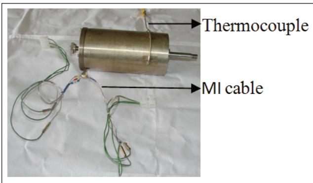
FIG. 11 LOW POWER INDUCTION MOTOR WITH MI CABLE
