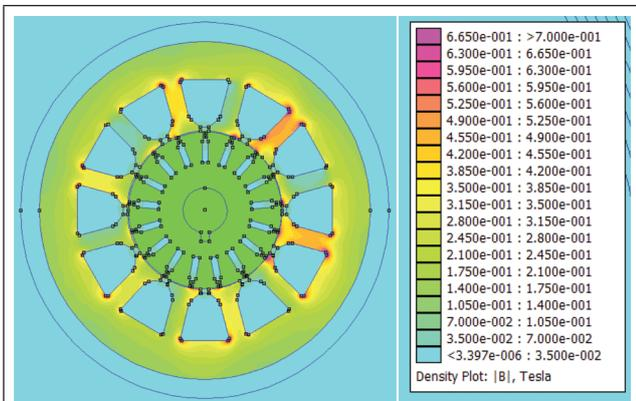
FIG. 16 MAGNETIC FLUX DENSITY PLOT IN STATOR (T)
