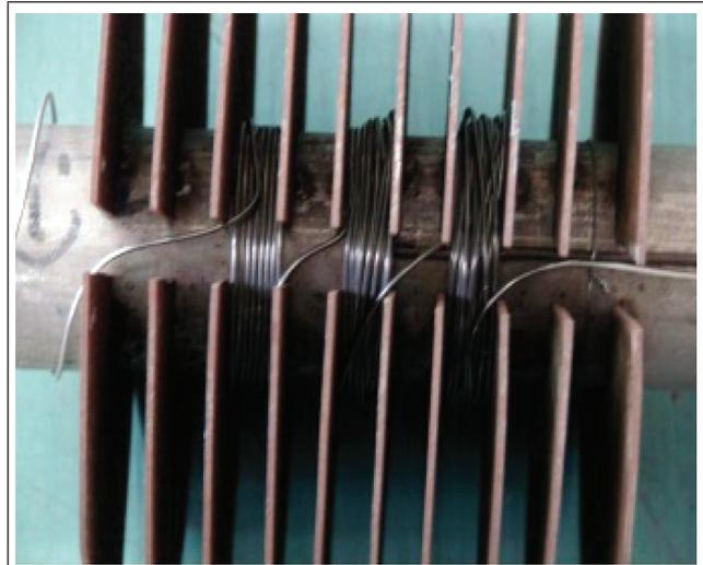
FIG. 7 MI CABLE IN WOUND CONDITION OVER A PIPE AND SLOT TYPE OF ARRANGEMENT
