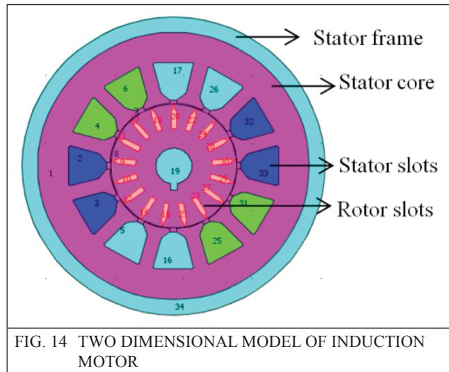
FIG. 14 TWO DIMENSIONAL MODEL OF INDUCTION MOTOR
