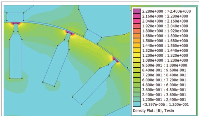
FIG. 17 MAGNETIC FLUX DENSITY PLOT IN ROTOR (T)
