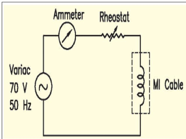
FIG. 6 SCHEMATIC OF TEST SET-UP FOR MI CABLE
