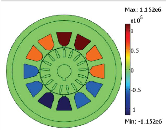
FIG. 15 EXTERNAL CURRENT DENSITY IN STATOR SLOT (A/MM<sup>2</sup>)
