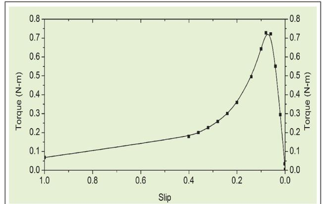
FIG. 18 TORQUE VERSES SLIP CHARACTERISTICS
