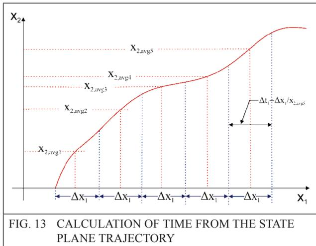
FIG. 13 CALCULATION OF TIME FROM THE STATE PLANE TRAJECTORY
