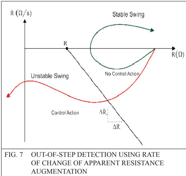
FIG. 7 OUT-OF-STEP DETECTION USING RATE OF CHANGE OF APPARENT RESISTANCE AUGMENTATION
