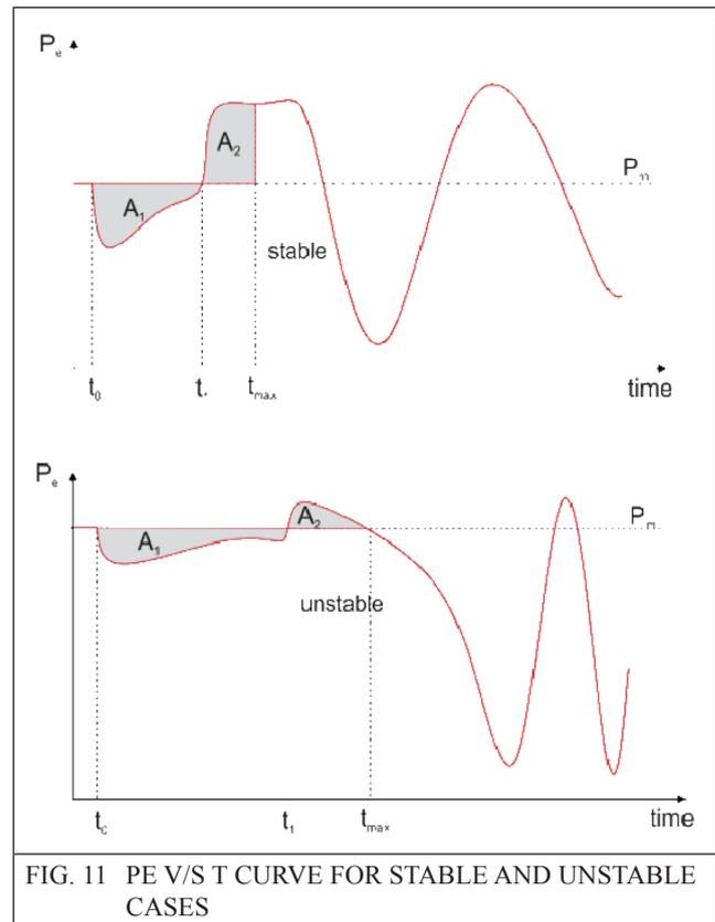
FIG. 11 PE V/S T CURVE FOR STABLE AND UNSTABLE CASES
