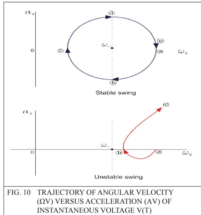
FIG. 10 TRAJECTORY OF ANGULAR VELOCITY ( $\Omega_V$ ) VERSUS ACCELERATION ( $\alpha_V$ ) OF INSTANTANEOUS VOLTAGE  $V(T)$
