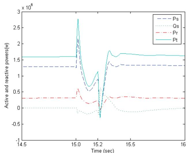
**Figure 3.** Stator active and reactive powers during fault duration of 15 to 15.2 sec<sup>7</sup>.
