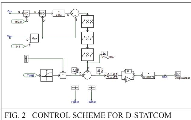
FIG. 2 CONTROL SCHEME FOR D-STATCOM
