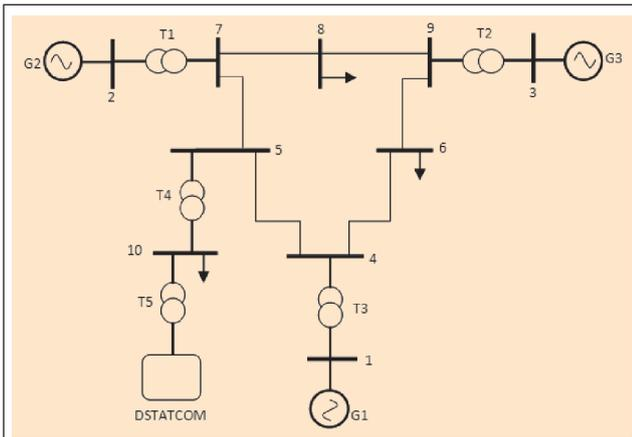
FIG. 1 SINGLE LINE DIAGRAM OF THE SYSTEM WITH D-STATCOM
