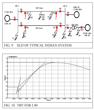
The TRV characteristic for short line fault (L90) for the typical Indian system is shown in Figure 10 above. The TRV peak (Uc) in this case was found to be 1592.1 kV peak and the RRRV was 3.99 kV/ $\mu$ s. For the case of transformer limited fault, the TRV peak and RRRV was found to be 1664.5 kV peak and 12.46 kV/ $\mu$ s respectively (Figure 11). These values are well within those specified by standards [2-3] i.e. 1799 kV peak for TRV and 16.1 to 18.0 kV/ $\mu$ s for RRRV.
