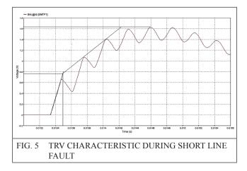
The test duties for SLF as per IEC are L90 and L75. Both IEEE and IEC require the SLF tests to be performed at 90 % and 75% of the rated short circuit current.
