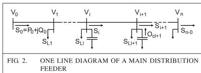
FIG. 2. ONE LINE DIAGRAM OF A MAIN DISTRIBUTION FEEDER
