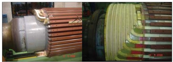
FIG. 4 PROCESS OF ROTOR REPAIRING
