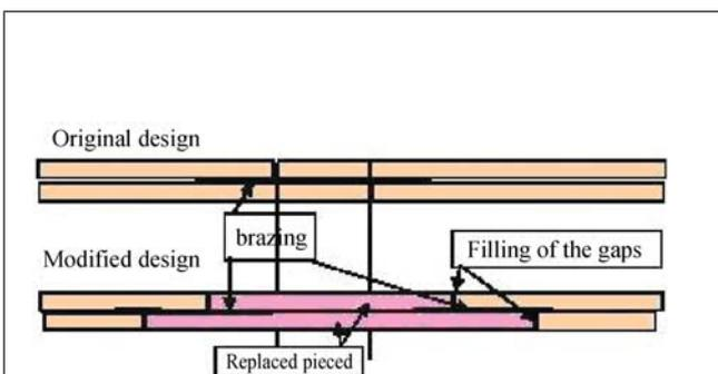
FIG. 12 COIL REPAIR AND REWIRED ROTOR
