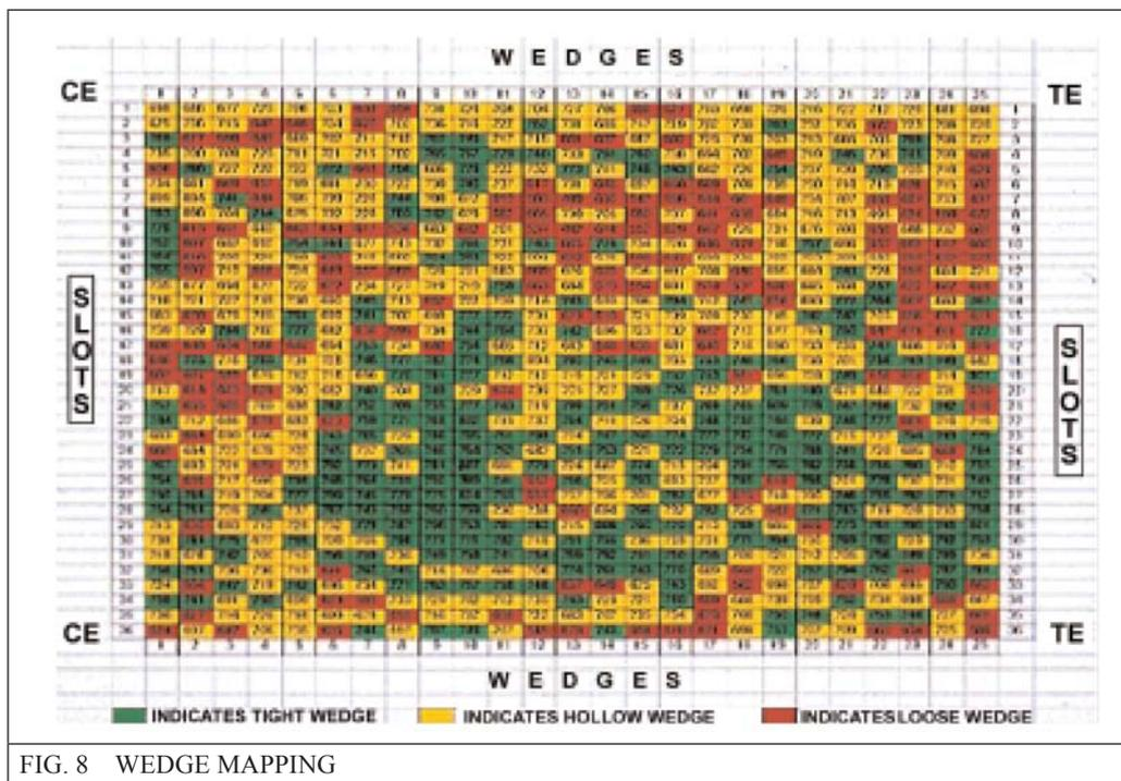
FIG. 8 WEDGE MAPPING
