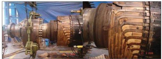
FIG. 3 DISASSEMBLY OF ROTOR
