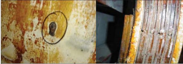
FIG. 10 INSULATION FAILURE AND CREATION OF VOID
