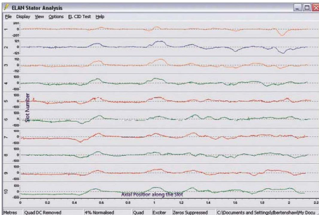
FIG. 7 ELCID TEST
