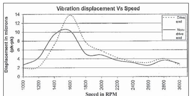
FIG. 5 VIBRATION DURING BALANCING
