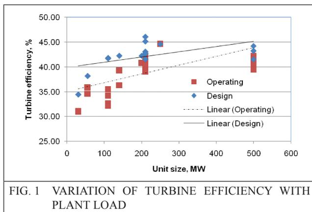
efficiency is large in smaller units of capacity 30–110 MW units, moderate in 210–250 MW units and minimal in 500 MW units. The trend shows the advances made in the design and due to aging of old smaller capacity units.
