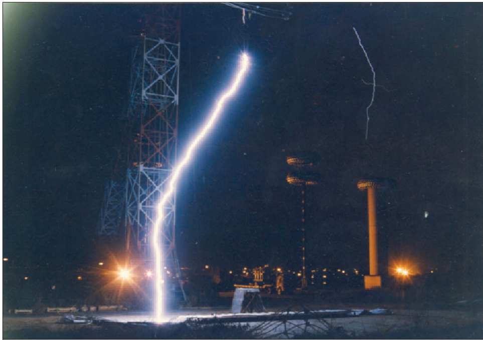
FIG. 2 A VIEW OF ROD-PLANE GAP FLASHOVER
