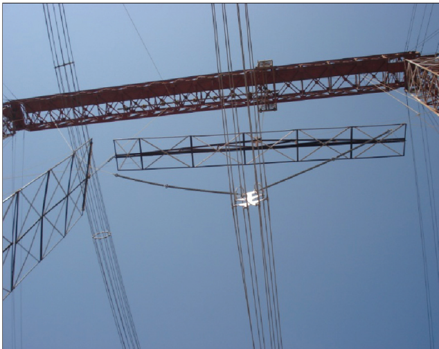
FIG. 10 SET UP FOR OBTAINING CRITICAL TIME TO PEAK FOR SWITCHING IMPULSE VOLTAGES
