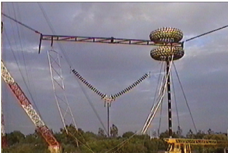
FIG. 6 A VIEW OF 400 kV STRING WITH TOWER SIDE SIMULATION FOR GAP FACTOR DETERMINATION
