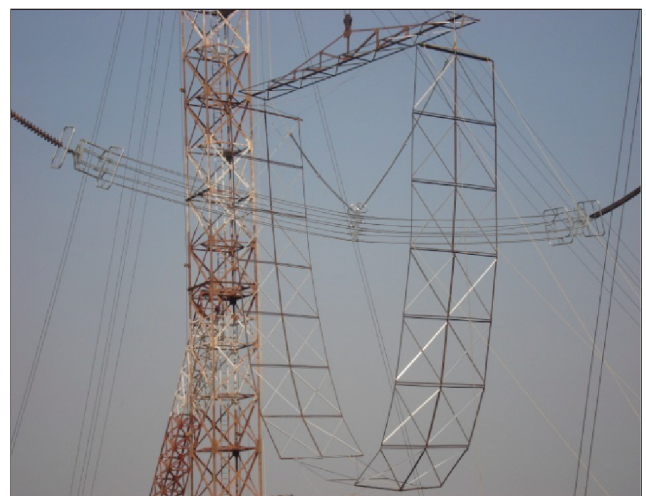
FIG. 12 THE ARRANGEMENT OF THE TOTAL SET UP WITH BUNDLE CONDUCTOR ALONG WITH INSULATOR STRING AND CONDUCTOR-TOWER WINDOW SIMULATION
