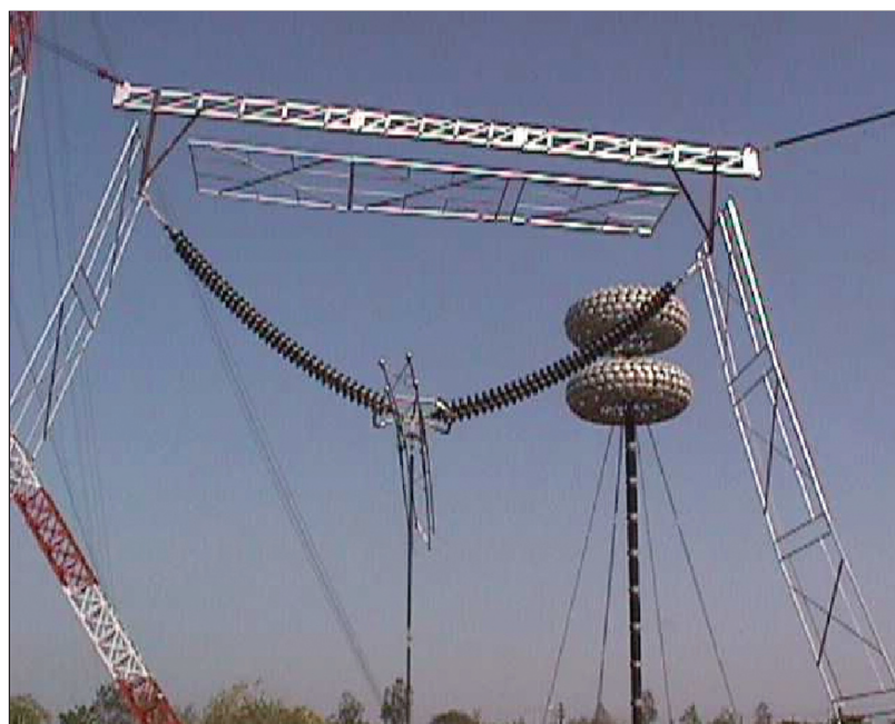
FIG. 7 A VIEW OF 800 kV INSULATOR STRING WITH SIMULATED TOWER
