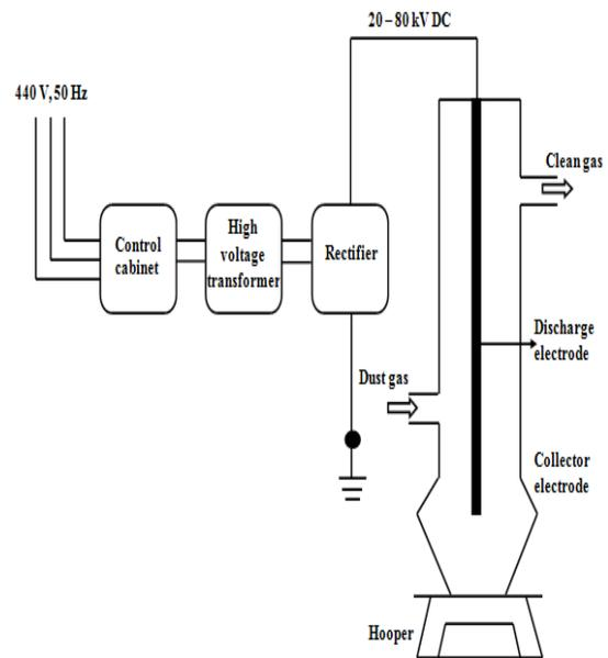
Figure 7. Electrostatic precipitator used for the removal of particulate matter.
