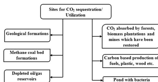
**Figure 4.** Sites for  $\text{CO}_2$  sequestration from a coal-fired thermal power plant.
