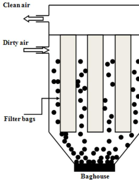
**Figure 8.** Baghouse fabric filter for the removal of larger particles.
