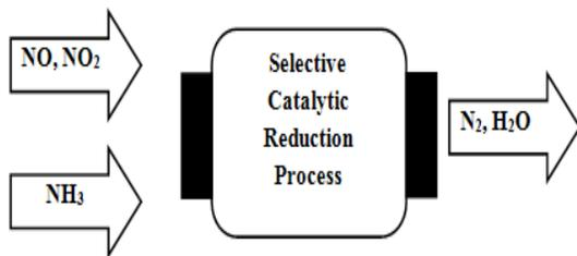
Figure 6. SCR for removal of NO<sub>x</sub>.
