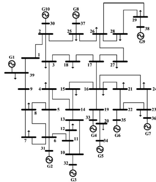
Figure 2. New England 39 Bus Test System.
