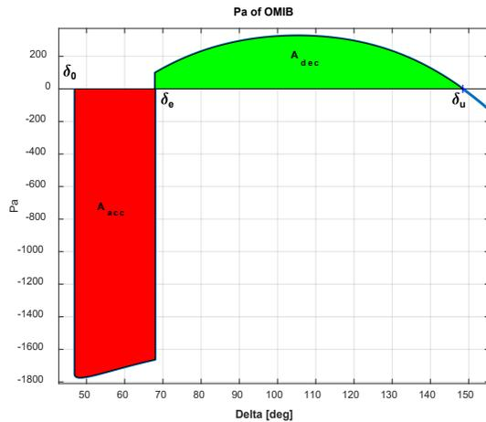
Figure 1. OMIB  $P_a$ - $\delta$  trajectory for an unstable case.
