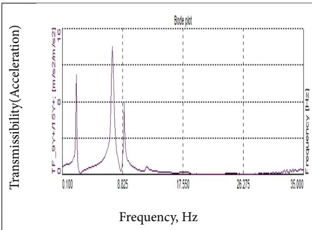
**Figure 3.** Resonance frequency (common base, transverse direction).
