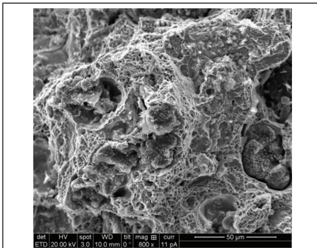
FIG. 7 SEM PHOTOGRAPH OF FRACTURED PMADI 1.5% Ni TENSILE SAMPLES AUSTEMPERED AT 340° C.
