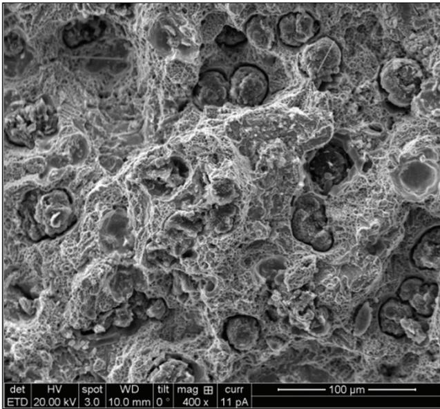
FIG. 9 SEM PHOTOGRAPH OF FRACTURED PMADI 2.5% Ni TENSILE SAMPLES AUSTEMPERED AT 340°C.
