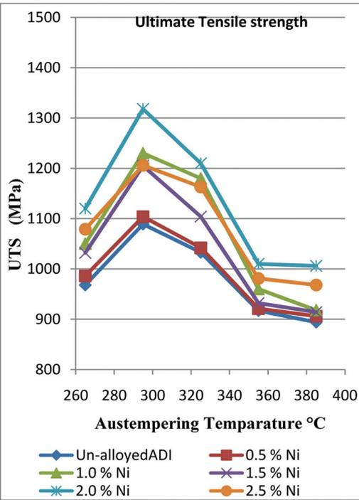
FIG. 10 TENSILE STRENGTH VARIATION WITH TWO-STEP AUSTEMPERING TEMP. AND % Ni.
