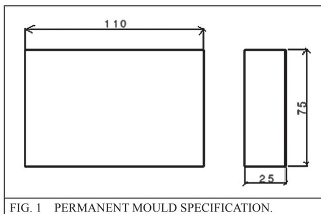
FIG. 1 PERMANENT MOULD SPECIFICATION.
