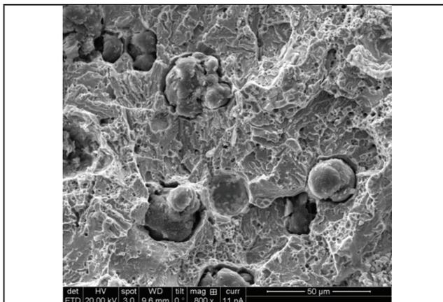
FIG. 8 SEM PHOTOGRAPH OF FRACTURED PMADI 2.0% Ni TENSILE SAMPLES AUSTEMPERED AT 340° C.
