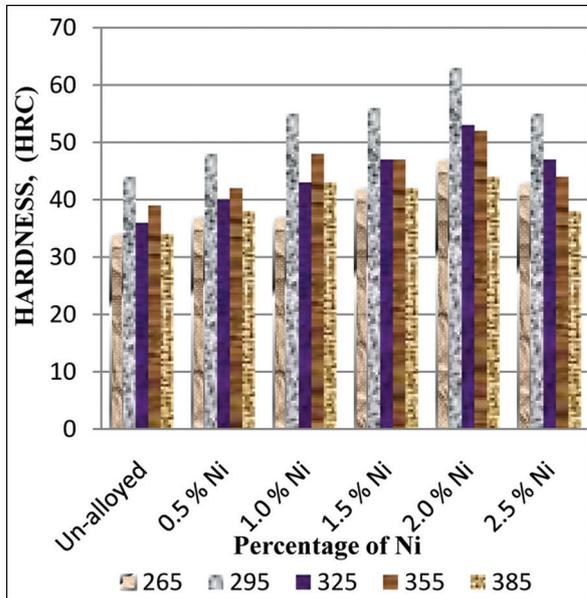
FIG. 12 HARDNESS VARIATION WITH TWO-STEP AUSTEMPERING TEMP. AND % Ni.
