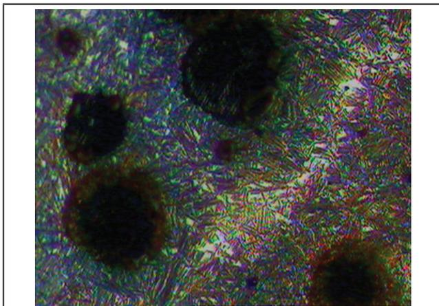
FIG. 4 MICROSTRUCTURE OF PMADI 1.5% Ni SAMPLES AUSTEMPERED AT 340° C (100X-NITAL ETCHED).
