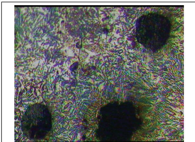
FIG. 5 MICROSTRUCTURE OF PMADI 2.0% Ni SAMPLES AUSTEMPERED AT 340° C (100X-NITAL ETCHED).
