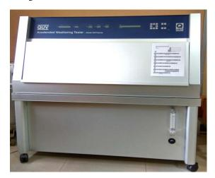
**Figure 1.** Accelerated weathering tester using fluorescent UV lamps.
