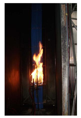
Figure 1. Flammability test on bunch of cables.
