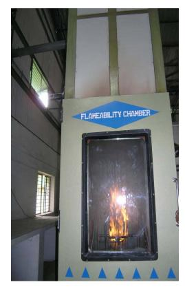
Figure 2. Flammability test chamber.
