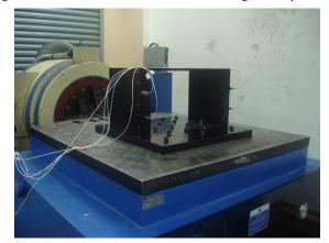
Figure 1. Typical fixture for relay mounting.
