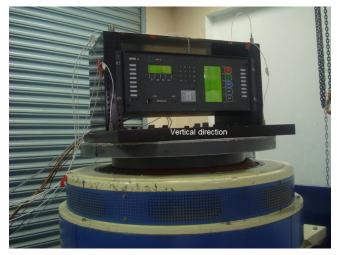
**Figure 2.** Relay test arrangement in three mutual perpendicular axes.
