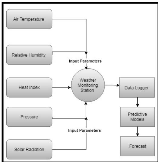
**Figure 4.** Simplified weather station signal-flow diagram.
