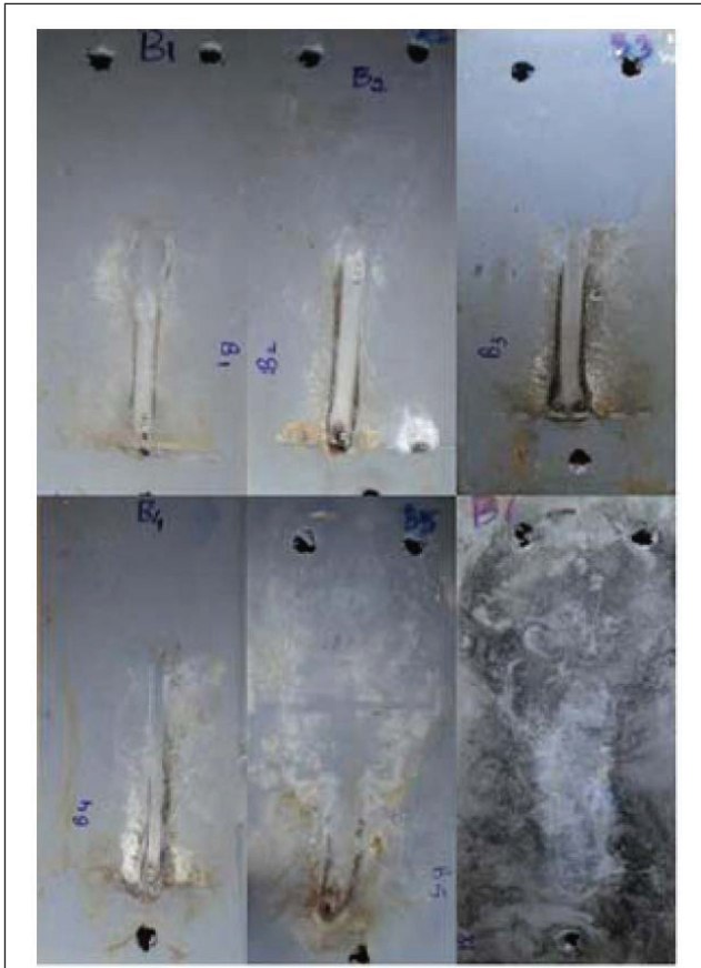
FIG. 4 PHOTOGRAPH OF IPTET SAMPLE OF FORMULATION B B1: ONLY IPTET B2: IPTET+UV 72.1 W/m 2 B3: IPTET+UV 49.3 W/m 2 B4: IPTET+UV23 W/m 2 B5: IPTET+UV72.1 W/m 2 +FLYASH B6: IPTET+UV72.1 W/m 2 +COAL
